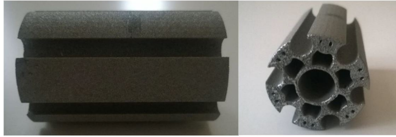
Figure 5.3: Illustration of an SLM-produced rotor [35]
