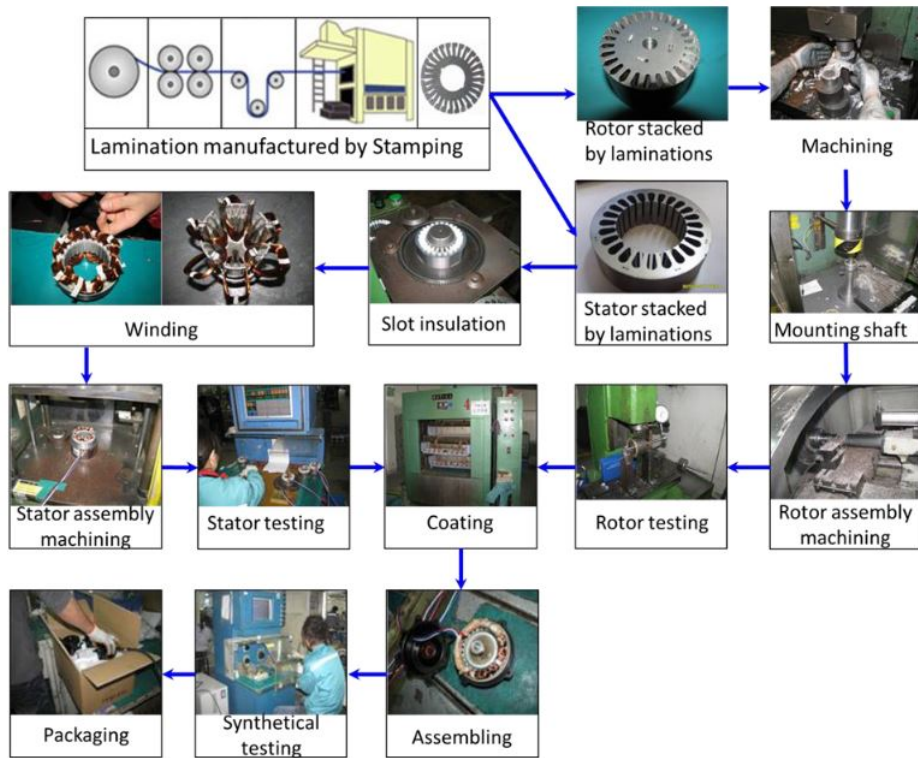
Figure 2.5: Overall process for traction electric motor production
