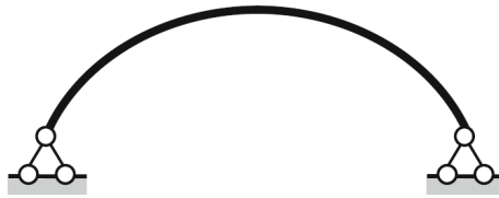
Figure 9.3: Two-Hinged Arch. Source [58]
