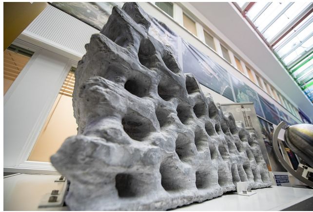
Figure 3.12: Structure obtained by 3D printing of lunar simulant, ESTEC
