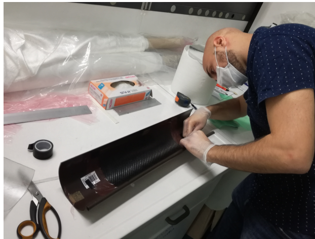
Figure 6.6: My colleague while making a Madflex curved panel.
