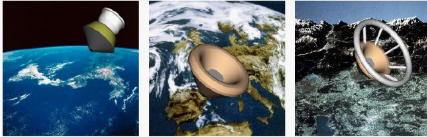
Figure 3.7. From the left: IRDT in orbital stored, re-entry and landing configuration
