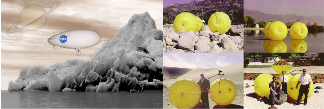
Figure 1.4. Titan aerover with inflatable wheels (left), inflatable rover concept vehicle (right)
