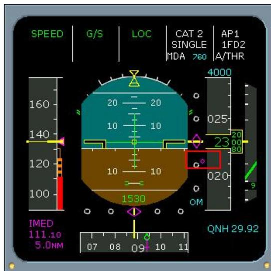
Figura 50: Primary Flight Display<sup>42</sup>
