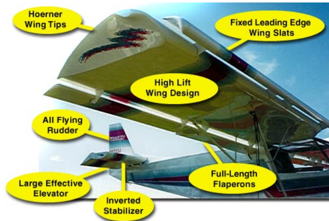
Figure 1.19: Wing and tail design of the Zenith CH 701 STOL, zenithair.net
