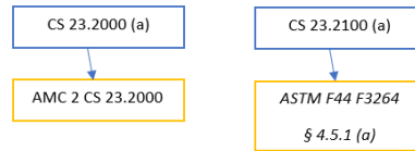
Figure 4.15: Example - Requirements traceability
