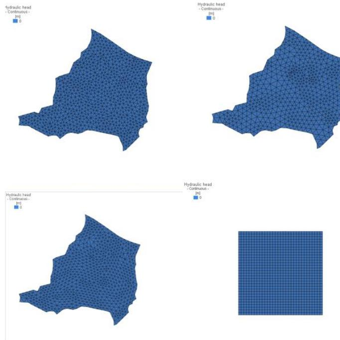
**Fig. 20.** Different types of mesh in FEFLOW (Triangle, Advancing Front, GridBuilder, Transport Mapping, respectively, from Top Left to Bottom Right)
