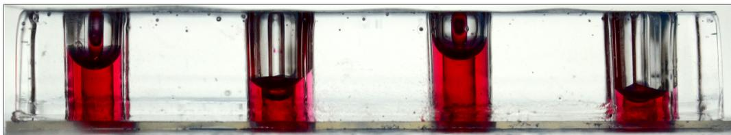
Figure 2.5. Case of capillary stop. Unequal liquid levels for a single unit at the end of the transitory, large inter-unit variability.
