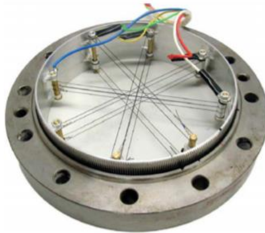
Figure 14 SMA-powered rotary harmonic drive system, Dilthey and Meier (2009).
