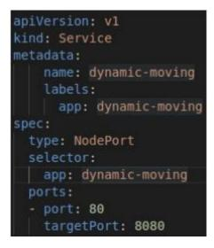
Figure 14 Service of the dynamic placement application
