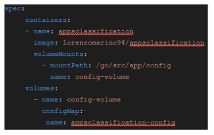
Figure 11 Volume mount for the ConfigMap inside pod definition
