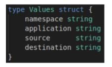
Figure 21 Structure to store the content of HTTP POST
