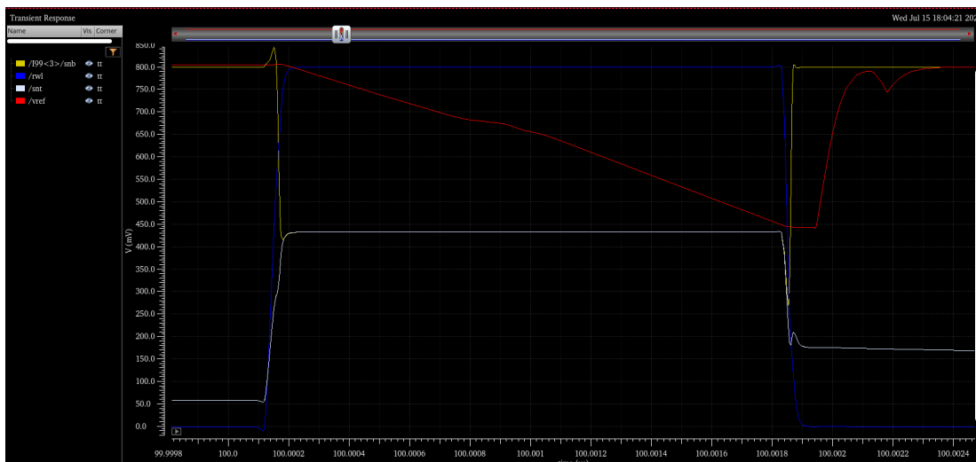
Figure 5.7: Waveform of voltage reference generator
