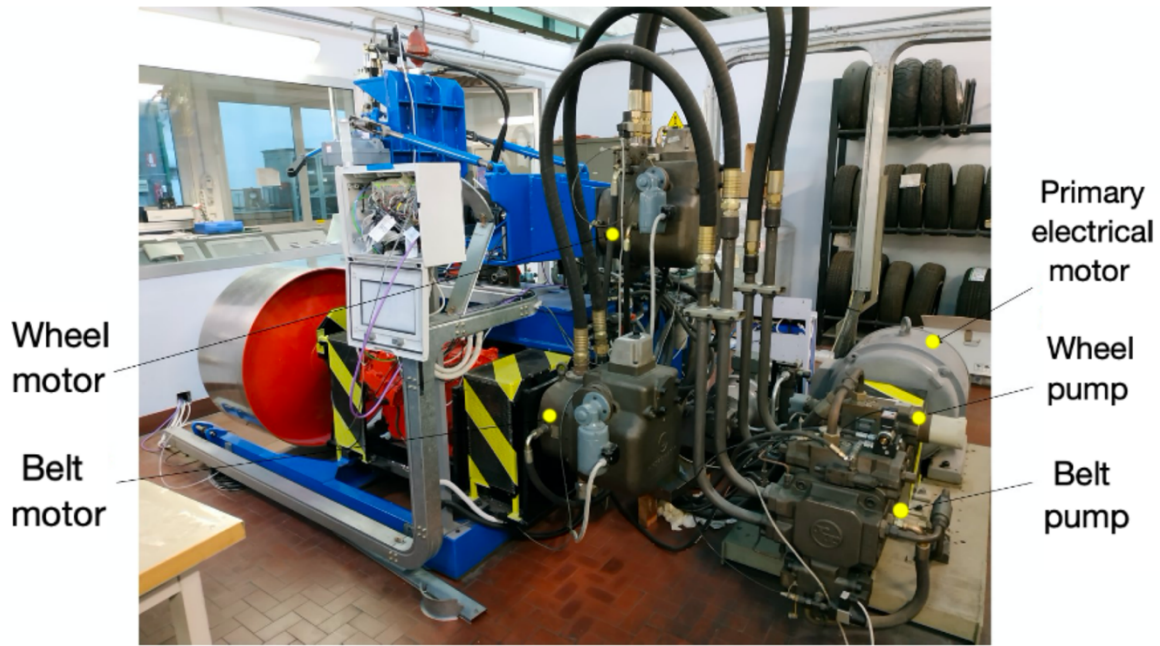
Fig. 1.10: Rear view of the Polito's tyre test bench
