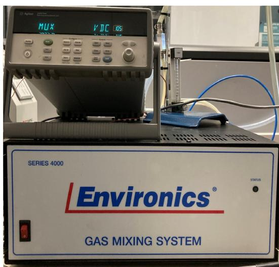
(c) Data logger (up) and gas mixing system (down).
