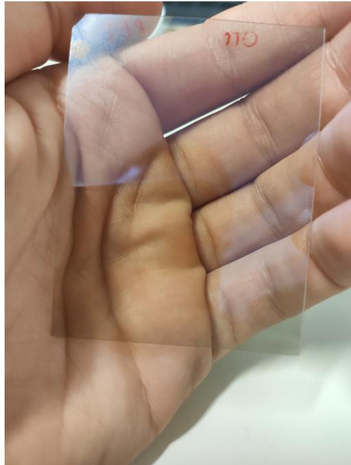
Figure 5.10: Conductive foil made of PET and ITO.
