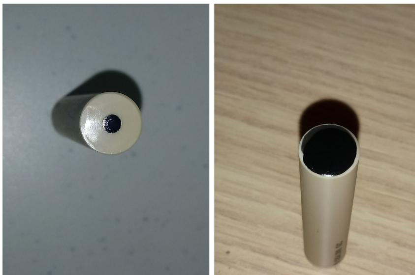
**Figure 6.2:** Glassy carbon electrode before and after the deposition of the slurry 3, obtained when using Nafion<sup>®</sup> resin solution as binder
