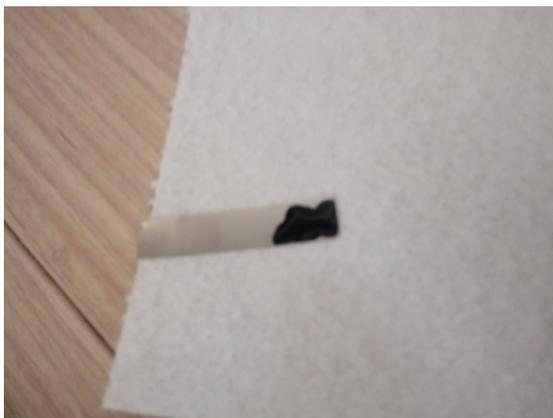
**Figure 6.3:** Electrode obtained when using Nafion<sup>®</sup> resin solution as binder, deposited on a titanium foil.
