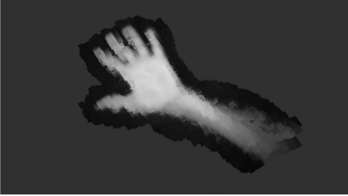
Figure 4.11: Representation of one hand in Rviz using PointCloud2 display
