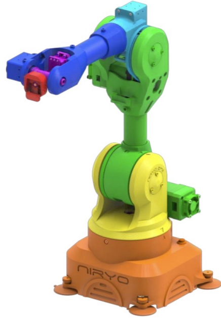
Figure 4.13: Niryo One structure composed of seven pieces, each one reported in the table on the left [48]
