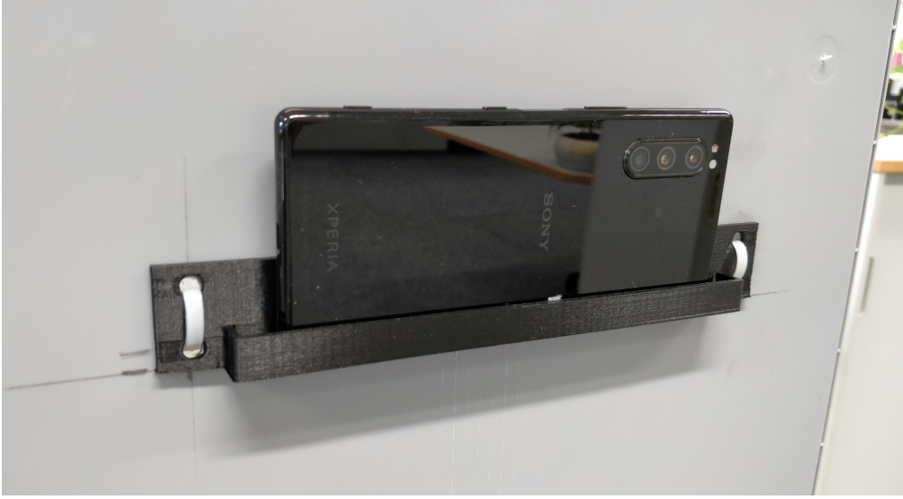
Figure 4.2: 3D-printed folder to locate the smartphone
