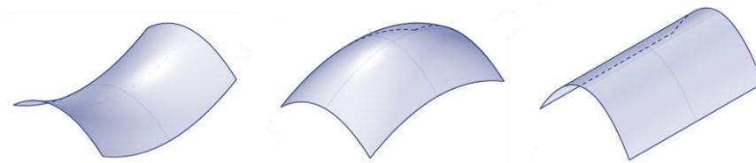
Fig. 3 Anticlastic, synclastic and monoclastic surfaces
