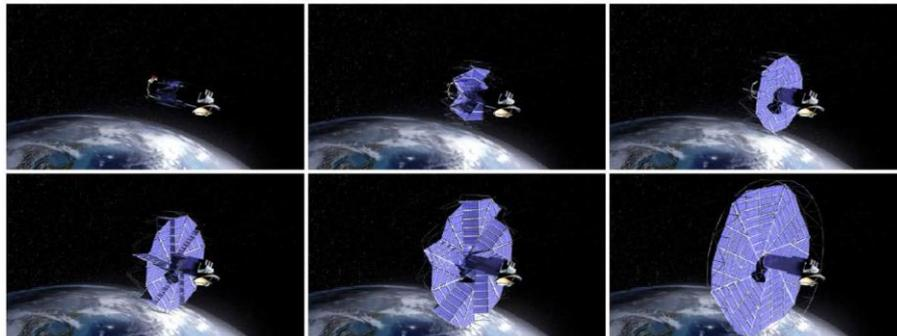
Fig. 48: A theoretical model of self-deployable solar panels using the principles of the Miura-Ori fold
