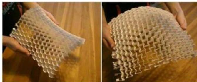
Fig. 4: Conventional material saddle shape and auxetic dome shape
