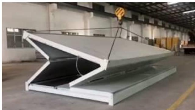
Fig. 50: Foldable container prototype
