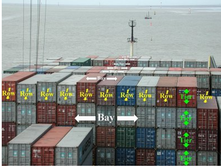
Figure 2.3: Container coordinates on a ship
