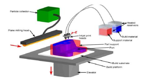
Fig. 3. Material Jetting process
