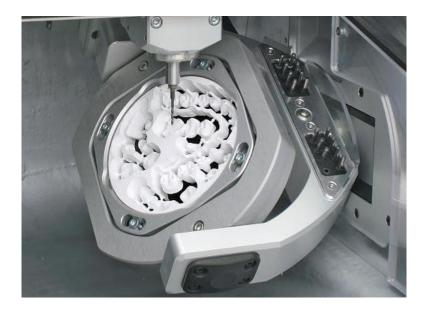
Fig. 39. Milling machine for dental applications
