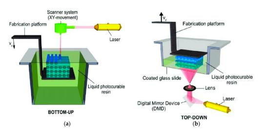
Fig. 9. Bottom-up approach (a) and Top-down approach (b)
