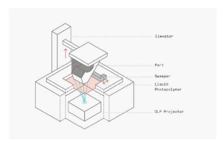
Fig. 8. Schematic of DPL printer
