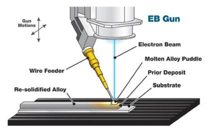
Fig. 11. Direct Energy Deposition
