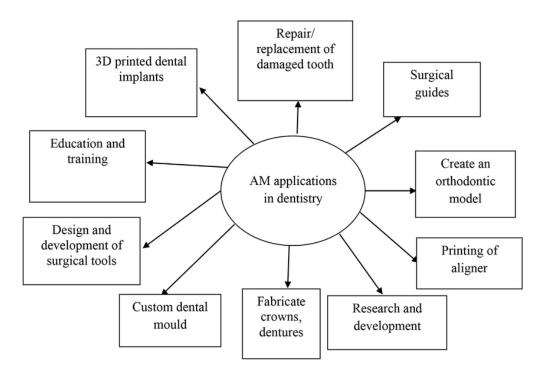
Fig. 40. Major additive manufacturing applications in Dentistry
