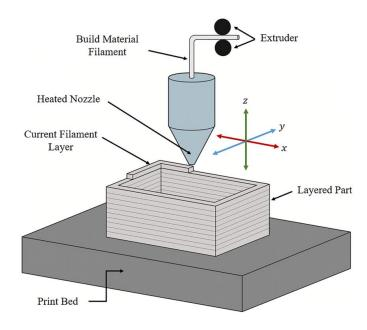
Fig. 2. Material Extrusion process
