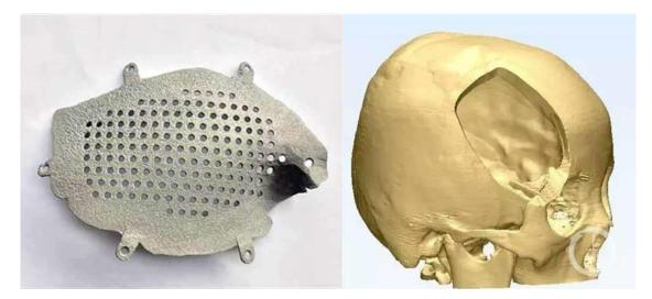
Fig. 21. 3D printed titanium prosthesis
