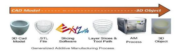
Fig. 1. Generalized Additive Manufacturing process
