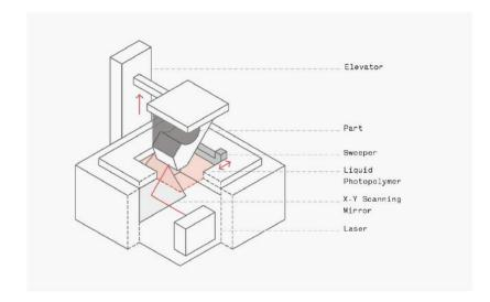
Fig. 7. Schematic of SLA printer
