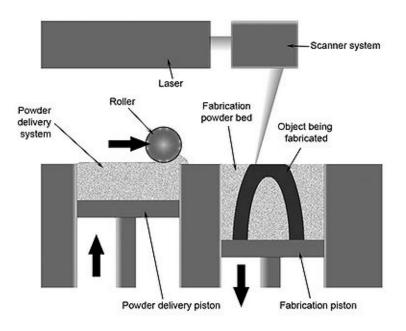
Fig. 10. Powder bed fusion process
