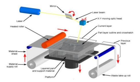
Fig. 5. Laminated object manufacturing
