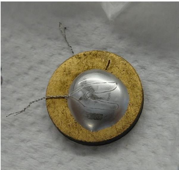
*Figure 2.9* – Gold sputtered sample with silver conductive paste coating and Pt wires
