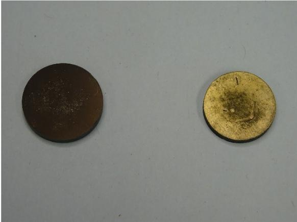
*Figure 2.8* – Picture of sintered gold sputtered samples: on the left, a scarcely densified sample, in which gold was partially internally absorbed; on the right, a sufficiently densified tablet
