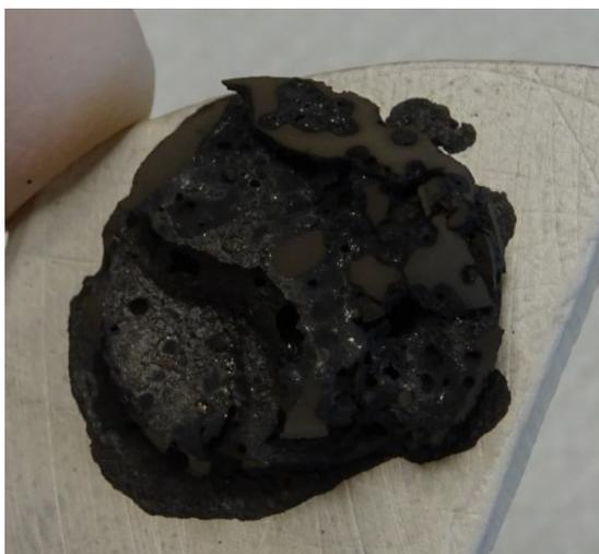
*Figure 4.25 – Sample of NFP material mixed with 10 %wt. of citric acid, sintered at 5 K/min to 560 °C, held for 3 hours, in Varigon atmosphere; here, laying on BN substrate*
