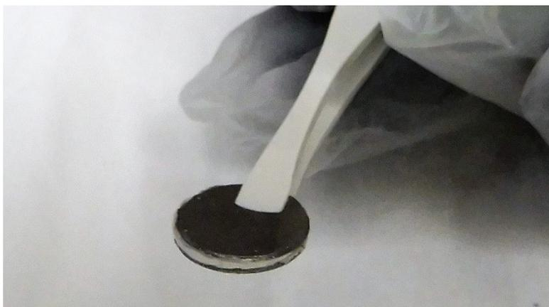
*Figure 3.5 – Picture of stacked sample in glovebox: the solid electrolyte (in the middle of the stack) has been coupled with metallic sodium and covered by graphite layers (in black)*
