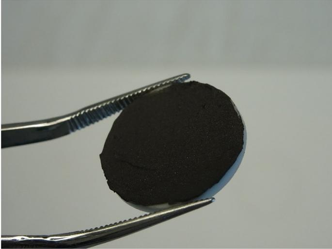
*Figure 3.7 – Picture of Na07 solid electrolyte, sintered with slurry of cathode material*
