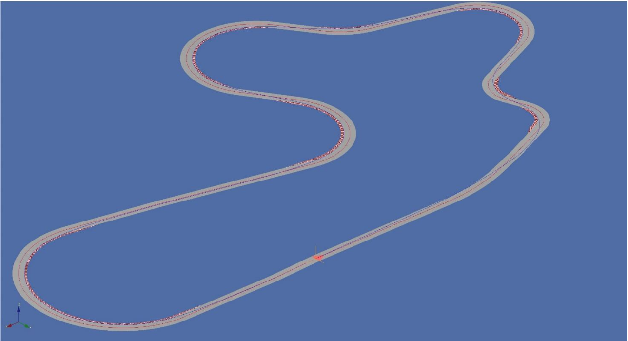
Figure 4.65 'Vi-Track' in Vi-Road with elevation profile, kerbs and bank angle in the corners. The blue path represents the driving line generated by the tool to optimize the vehicle performances, while the red path is the track centreline.
