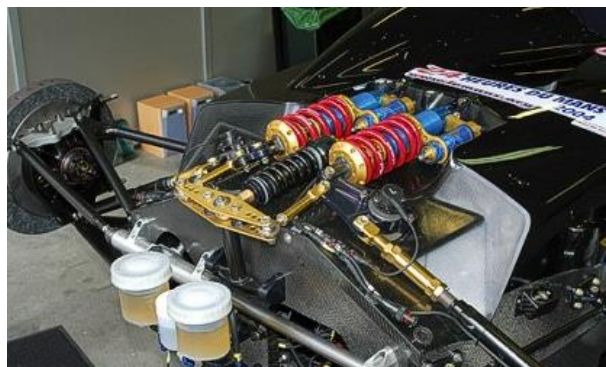
Fig 6a) A typical F1 heave spring-damper installation with disc spring elements, Red Bull F1 team 2019 [7]; 6b) A third spring-damper (black) actuated by rods and rocker arm mechanism [8].
