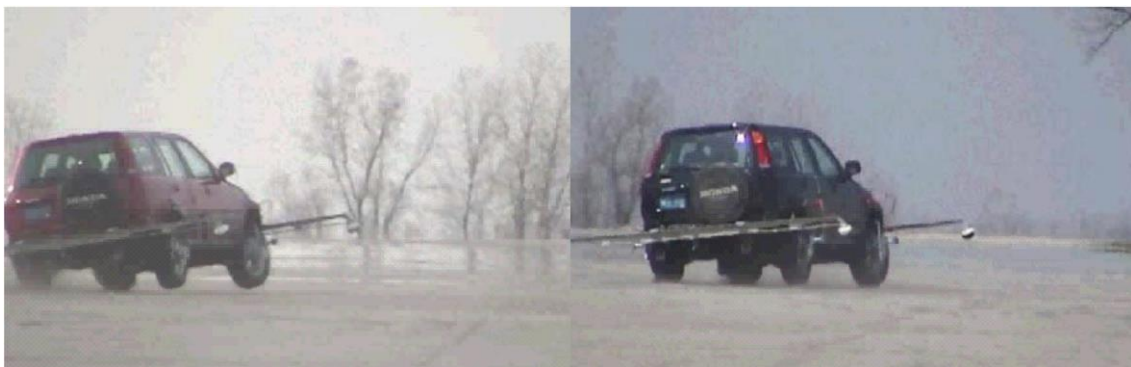
Fig. 23) Photo taken from the experimental test, illustrating the differences during standard Fishhook manoeuvre between the standard vehicle (on the left) and the Kinetic vehicle (on the right) [25].
