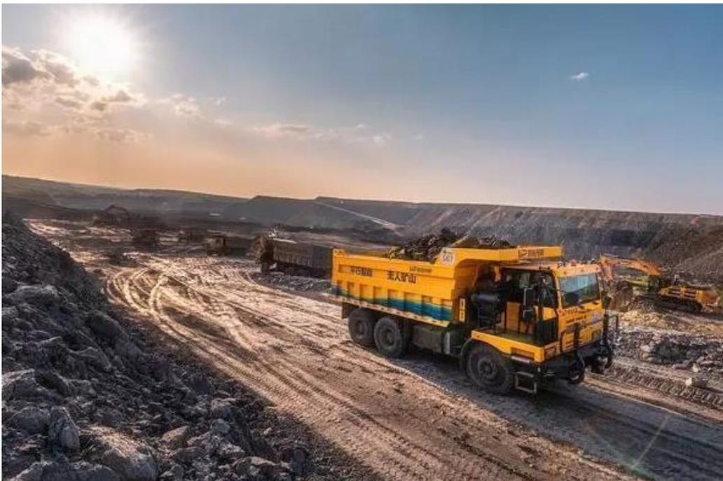
Figure 1.4 Autonomous Minecart
