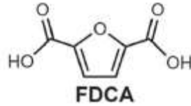
Figura 2.1: Molecola di FDCA. Si possono notare i due gruppi carbossilici -COOH ai due lati dell'anello furanico. (Sajid M., Zhao X., Liu D., 2018, Production of 2,5-furandicarboxylic acid (FDCA) from 5-hydroxymethylfurfural (HMF): recent progress focusing on the chemical-catalytic routes, Green Chem. , 20, 5427–5453. [DOI:10.1039/c8gc02680g]).
