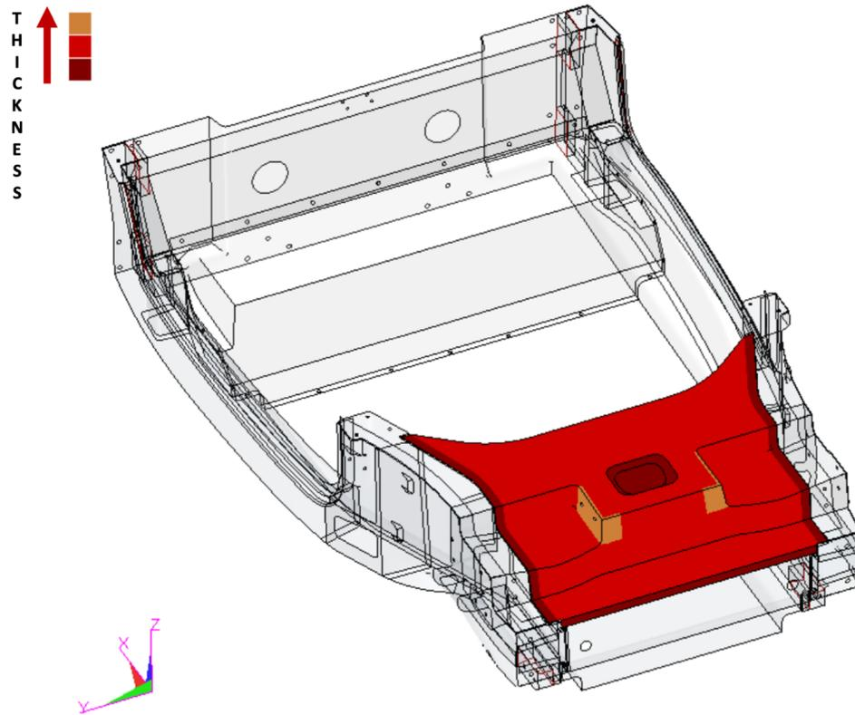
**Figure 3.7:** Front bulkhead layup
