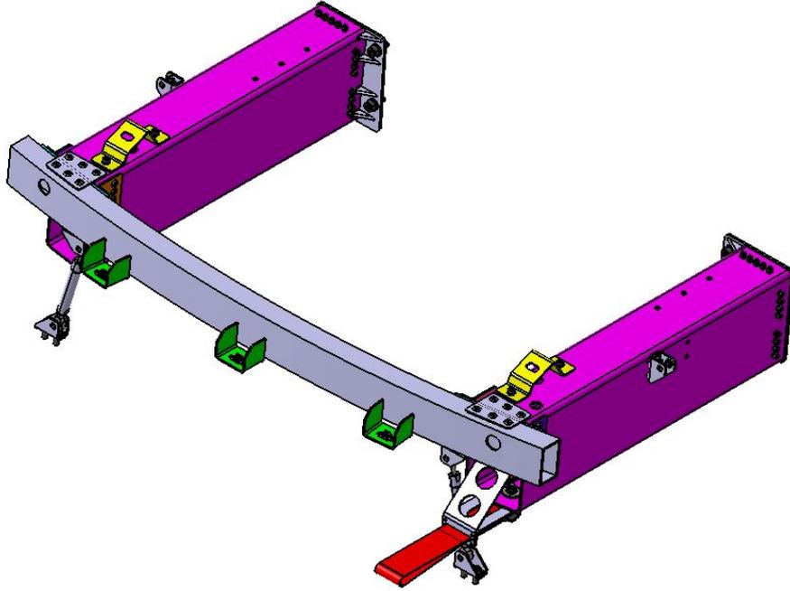
**Figure 4.1:** 3D model of the front crash structure
