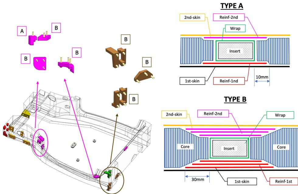
Figure 3.13: Front crash structure lamination scheme
