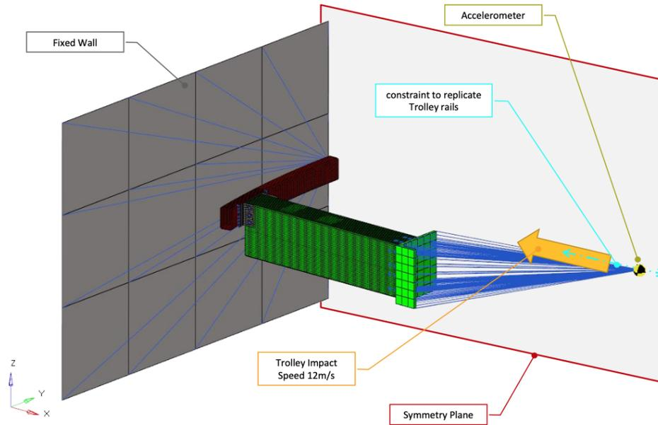
**Figure 4.2:** Front crash structure FEA model
