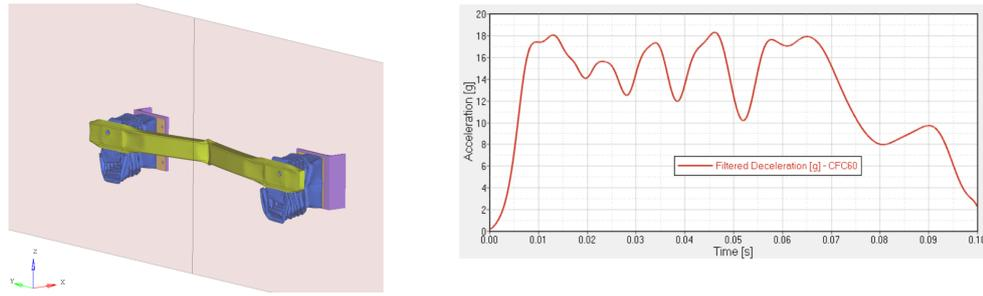
**Figure 4.3:** Crashed 3mm components at the end and deceleration vs time graph
