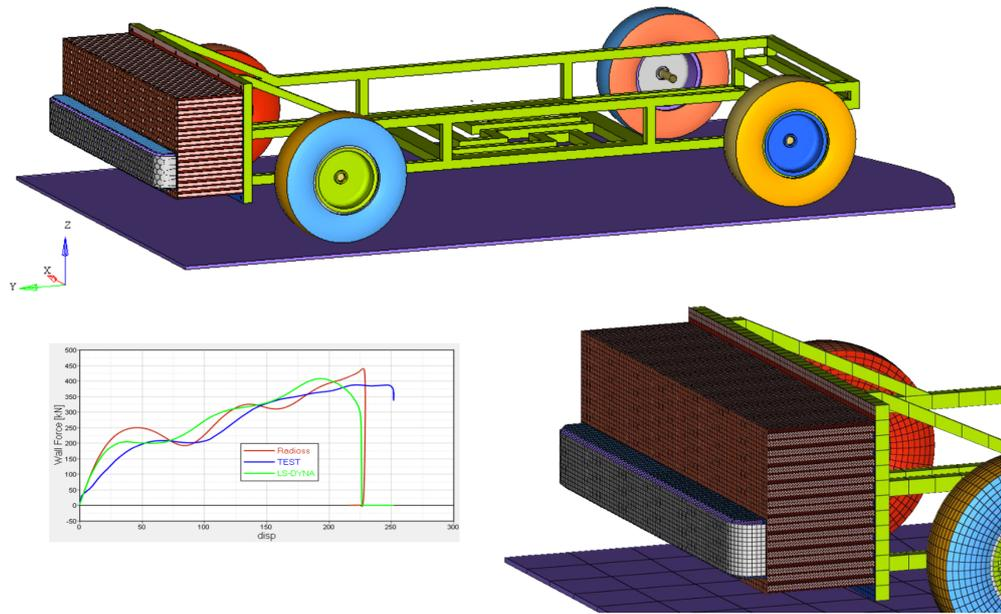
**Figure 4.14:** Movable test barrier
