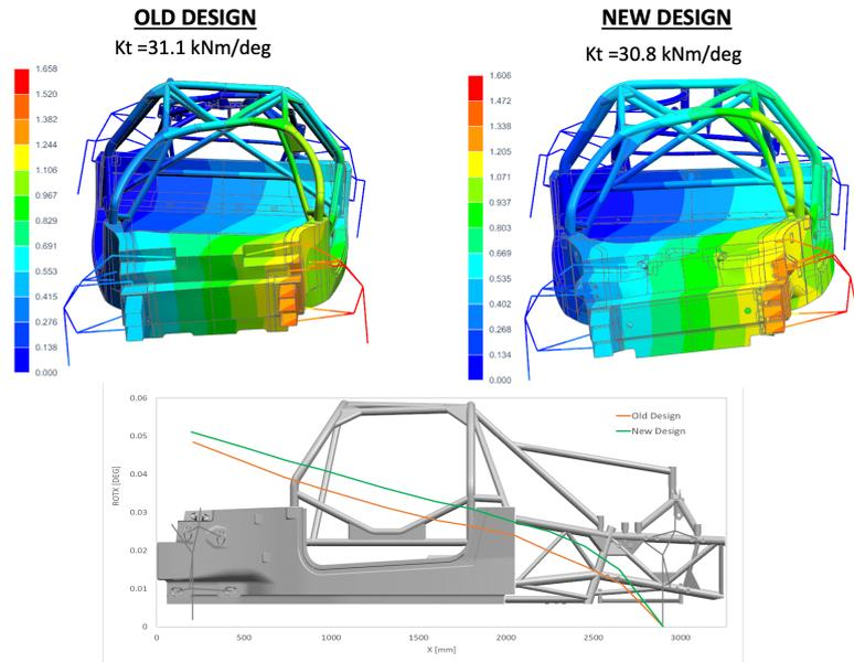
Figure 4.19: Torsional stiffness: 1<sup>st</sup> and 2<sup>nd</sup> run
