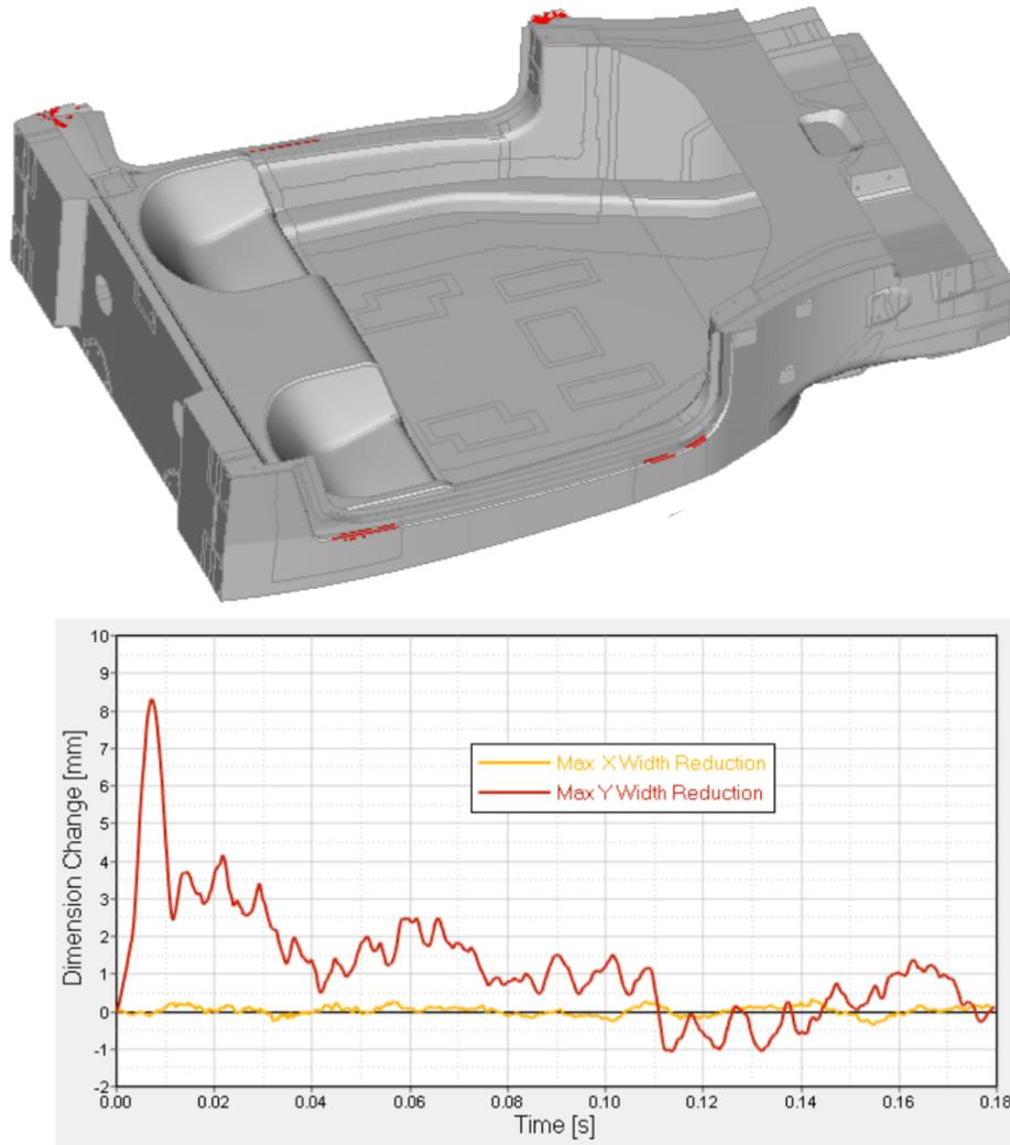
**Figure 4.17:** Side crash: damage results
