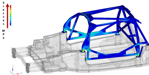
Figure 4.7: Front crash impact: roll-cage stresses
