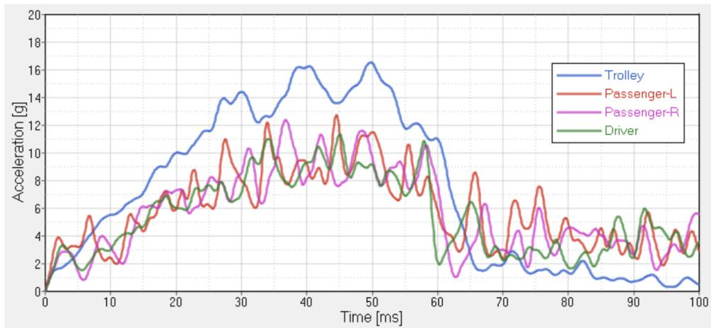
**Figure 4.16:** Side impact test: accelerations
