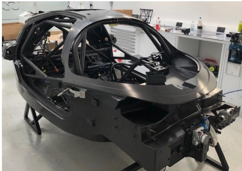
**Figure 5.9:** The finished cockpit structure
