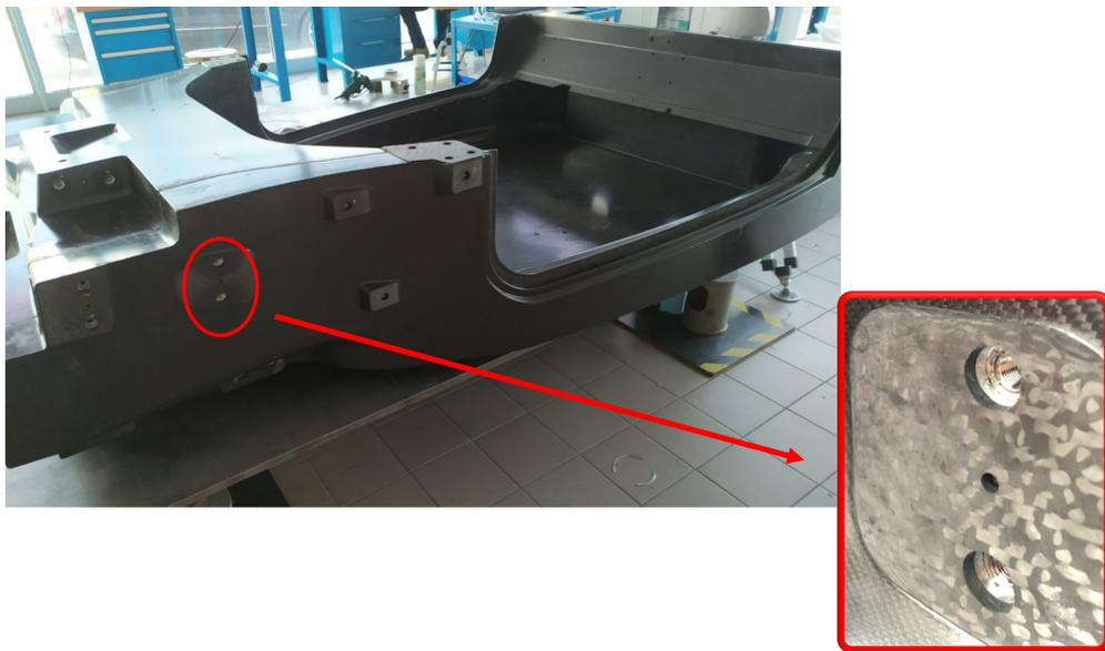
**Figure 5.3:** Monocoque machining details
