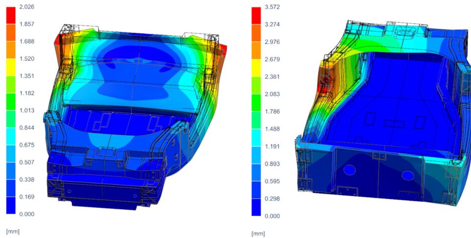
**Figure 4.13:** Monocoque deformations: main hoop and front hoop test
