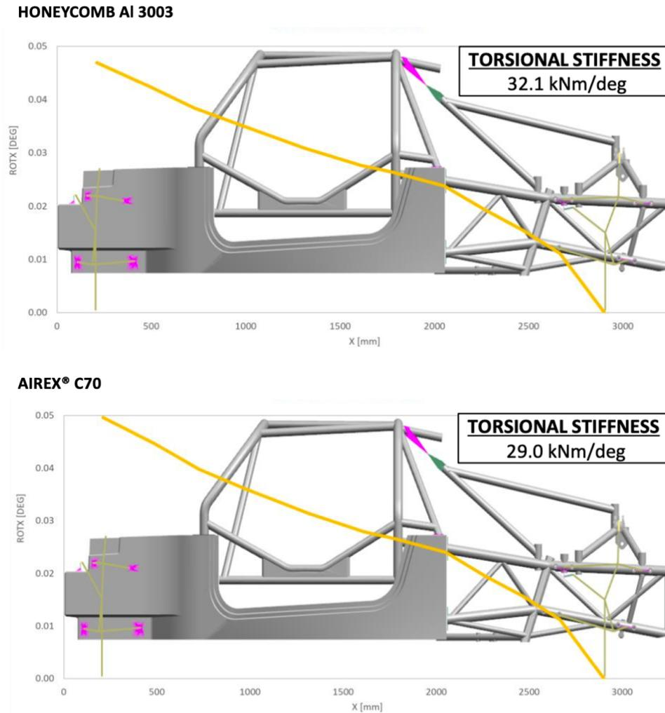
**Figure 3.3:** Honeycomb vs Airex<sup>®</sup> torsional stiffness comparison
