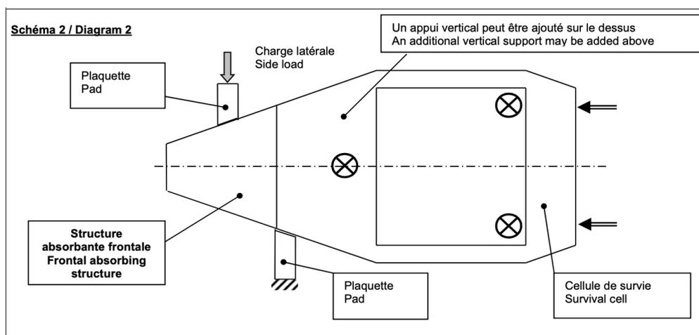
Figure 2.2: Front crash: test setup
