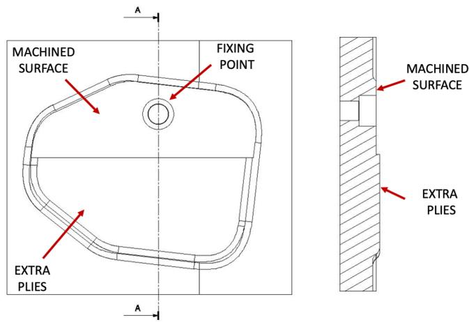
**Figure 3.2:** Machined planar surface
