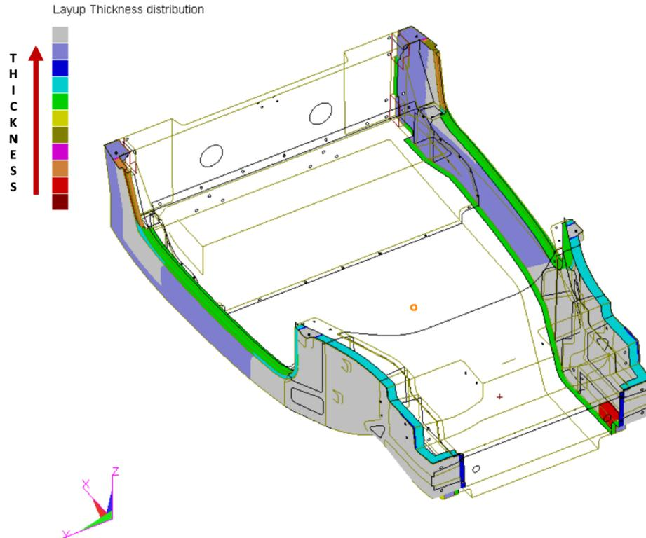
**Figure 3.4:** Door sill layup thickness
