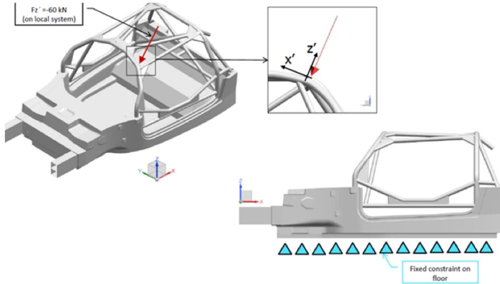
Figure 4.9: Front hoop test
