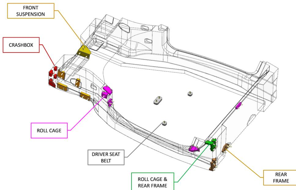
**Figure 3.8:** Insert positions in half car
