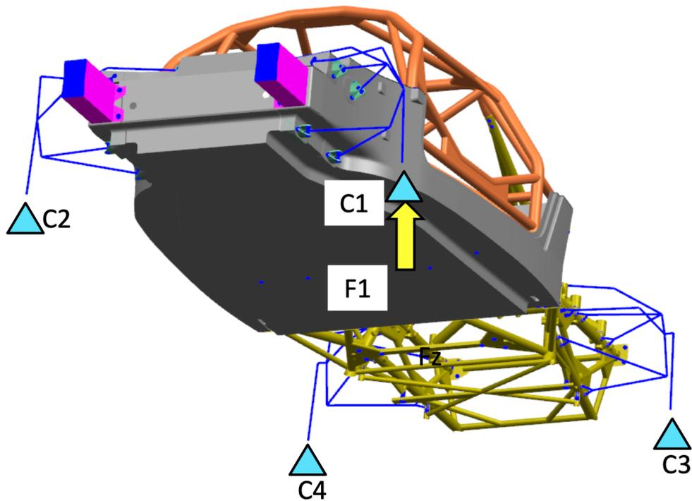
**Figure 4.18:** Torsional stiffness test setup
