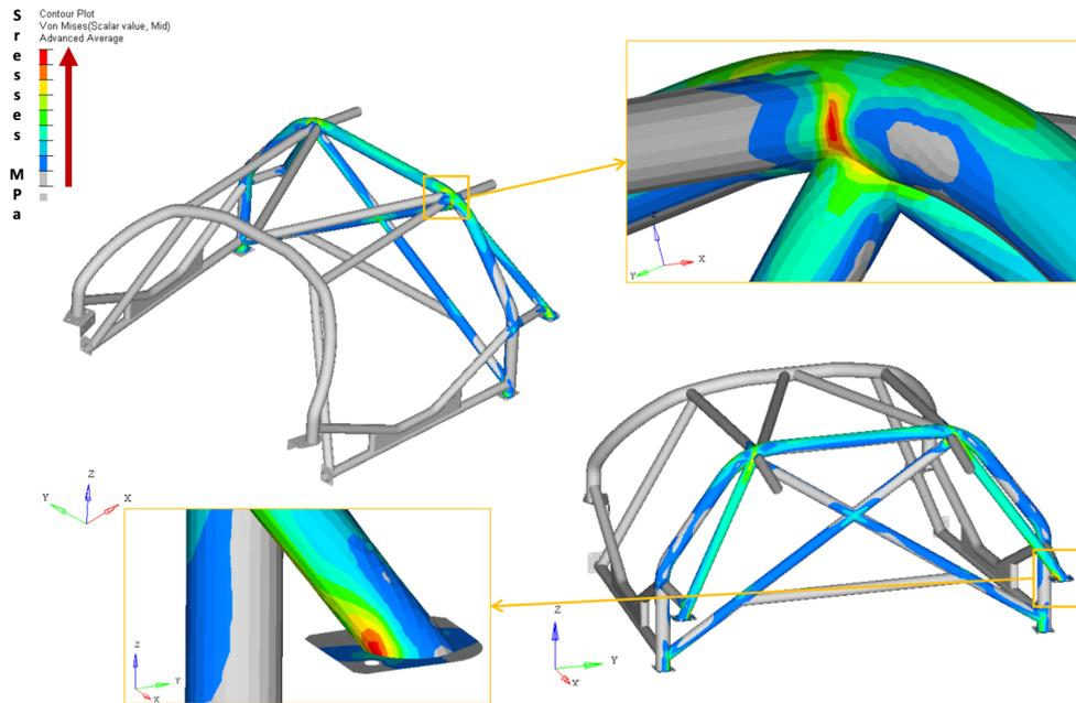
**Figure 4.10:** Main hoop test stresses
