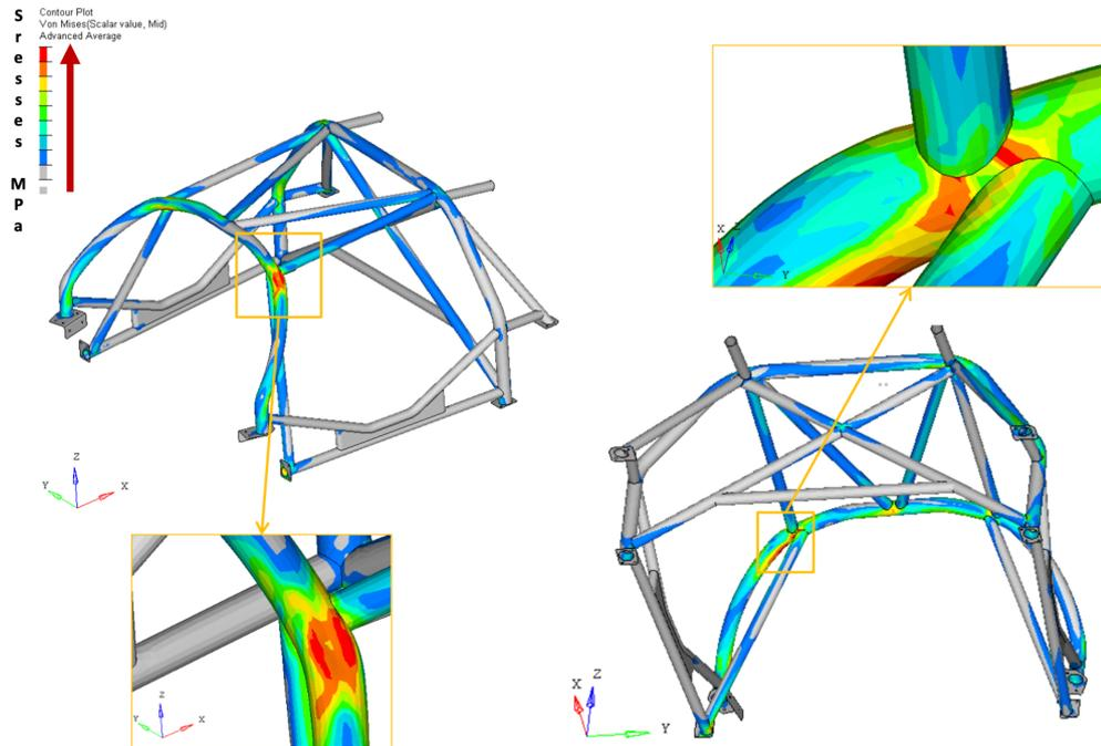
Figure 4.11: Front hoop test stresses
