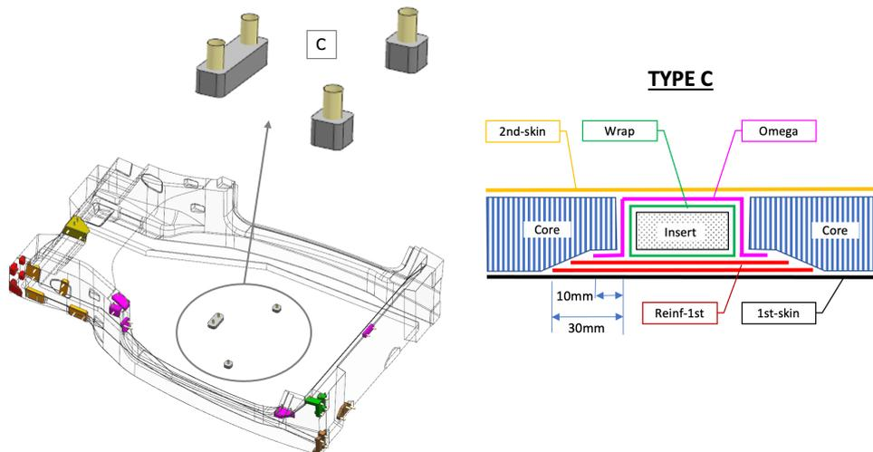
Figure 3.14: Front crash structure lamination scheme
