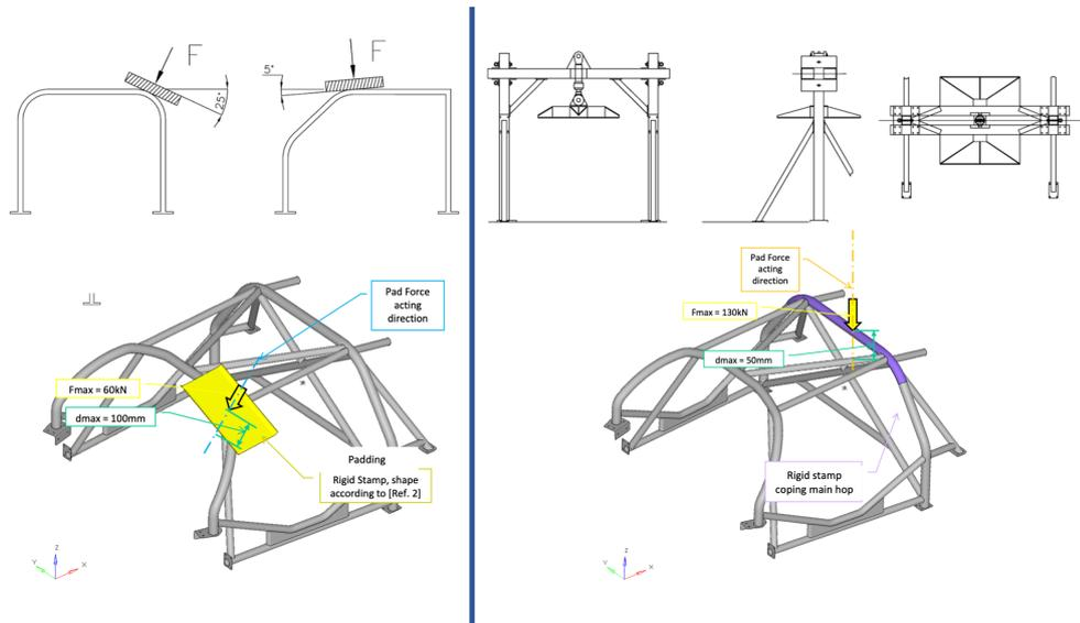
Figure 2.3: Front hoop and main hoop test rigs
