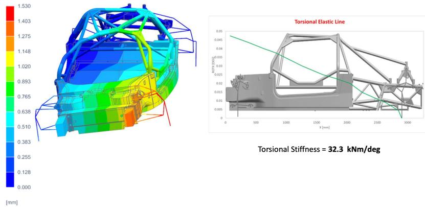
Figure 4.20: Torsional stiffness: final value
