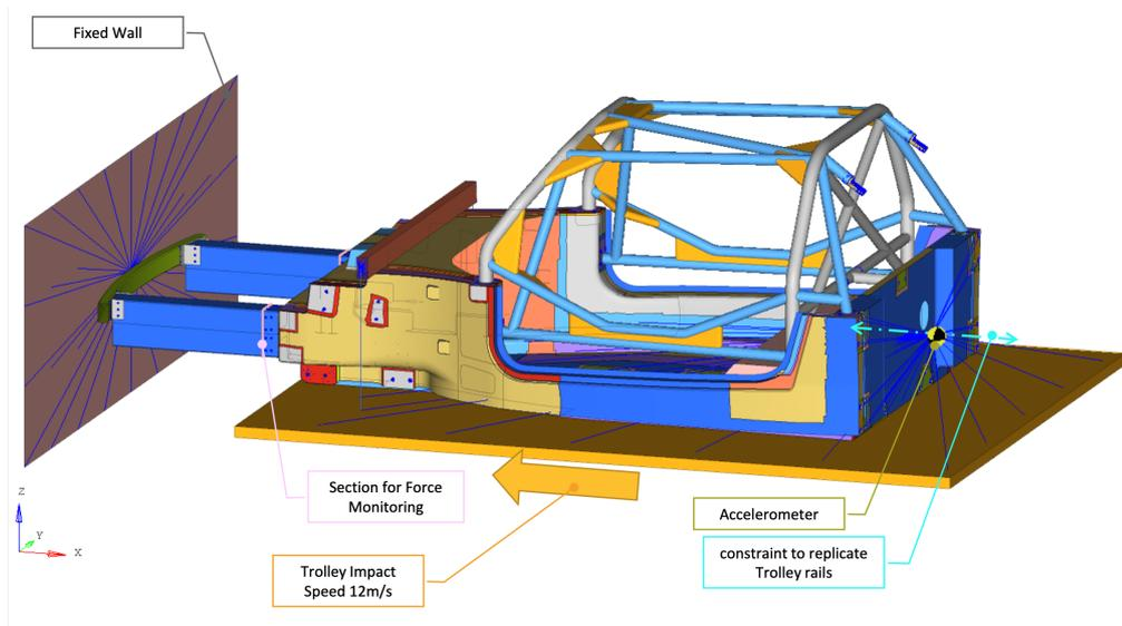
**Figure 4.4:** Chassis FEA model for front crash
