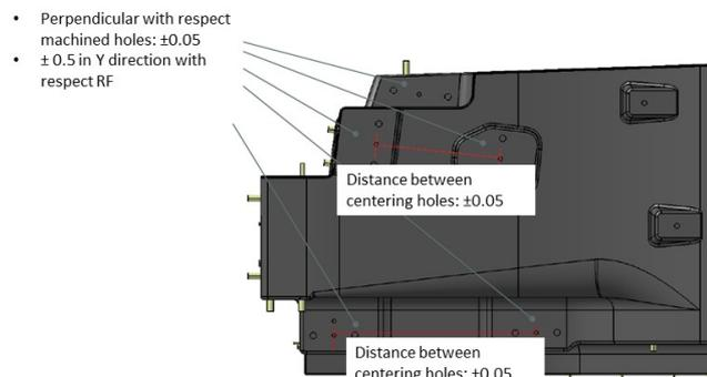
**Figure 5.4:** Accepted tolerances on monocoque machining
