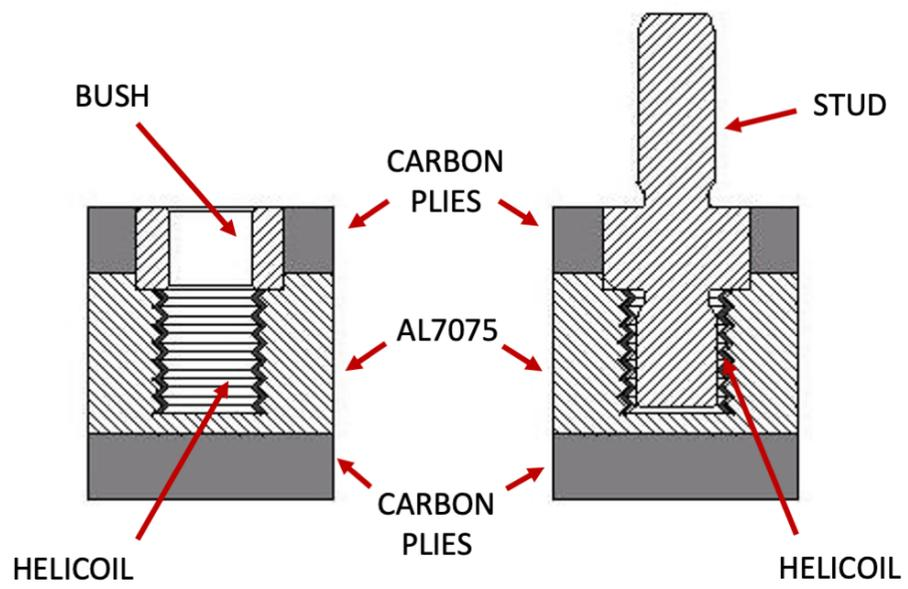
**Figure 3.16:** Inserts machining details
