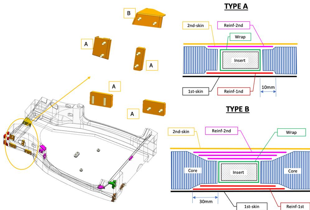
**Figure 3.10:** Front suspension insert lamination scheme
