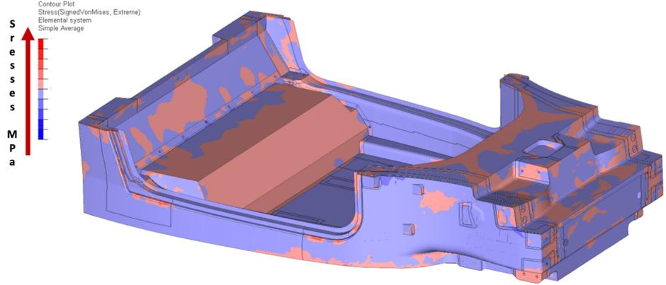
**Figure 4.5:** Front crash impact: monocoque stresses
