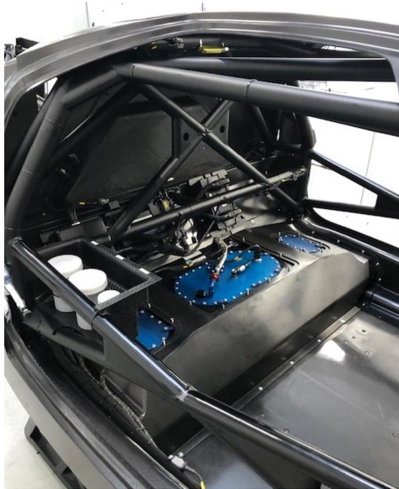
**Figure 5.8:** Fuel cell assembled inside the cockpit
