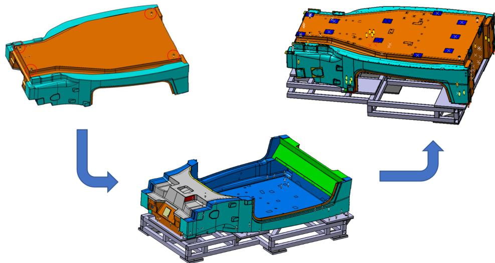
**Figure 5.2:** Monocoque machining phases
