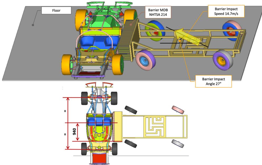
**Figure 4.15:** Side crash test setup
