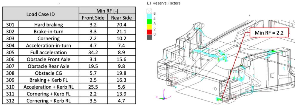
Figure 2.4: Load case for the chassis design
