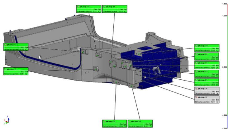
**Figure 5.5:** Planarity surface measurements
