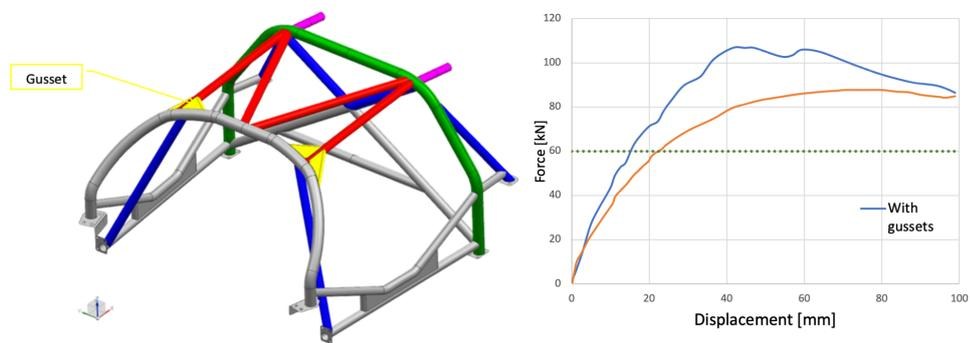
Figure 4.12: Front hoop behaviour with gussets and no gussets
