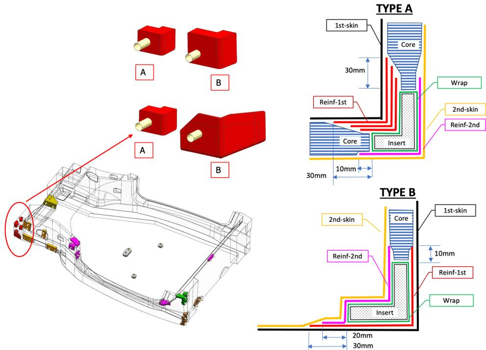
**Figure 3.12:** Front crash structure lamination scheme
