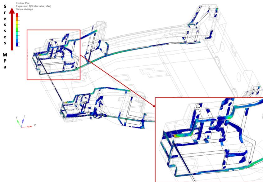
Figure 4.6: Front crash impact: glued surfaces stresses
