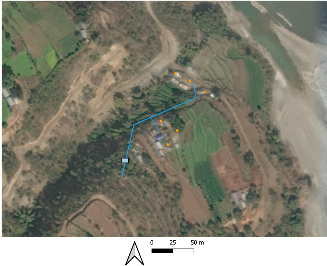
Figure 4: Satellite image. Note three sub-groups of households (one for each sub-branch of the main pipe).
