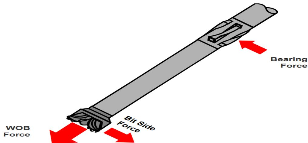
Figure 2-7 Pendulum principle(Rabia, 2002)
