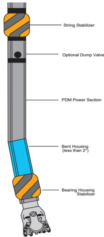
Figure 2-5 Steerable motor (Schlumberger, 1996)
