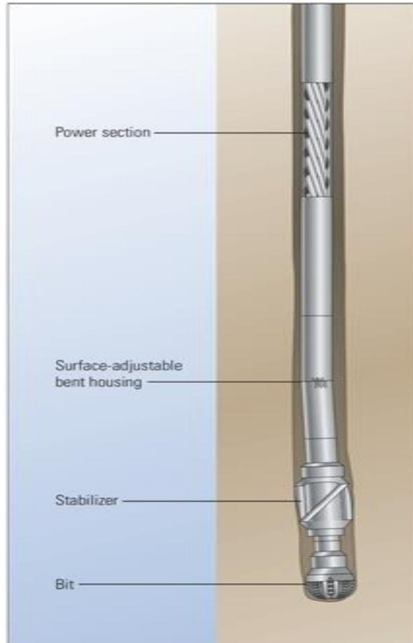
Figure 3-9 Conventional mud motor (Felczak et al., 2011)
