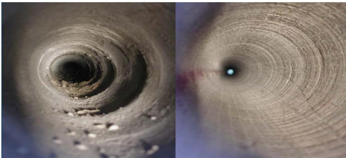
Figure 4-8 Comparison in the hole quality "push-the-bit" on (left) and "point-the-bit" techniques on (right).(Williams, 2006)
