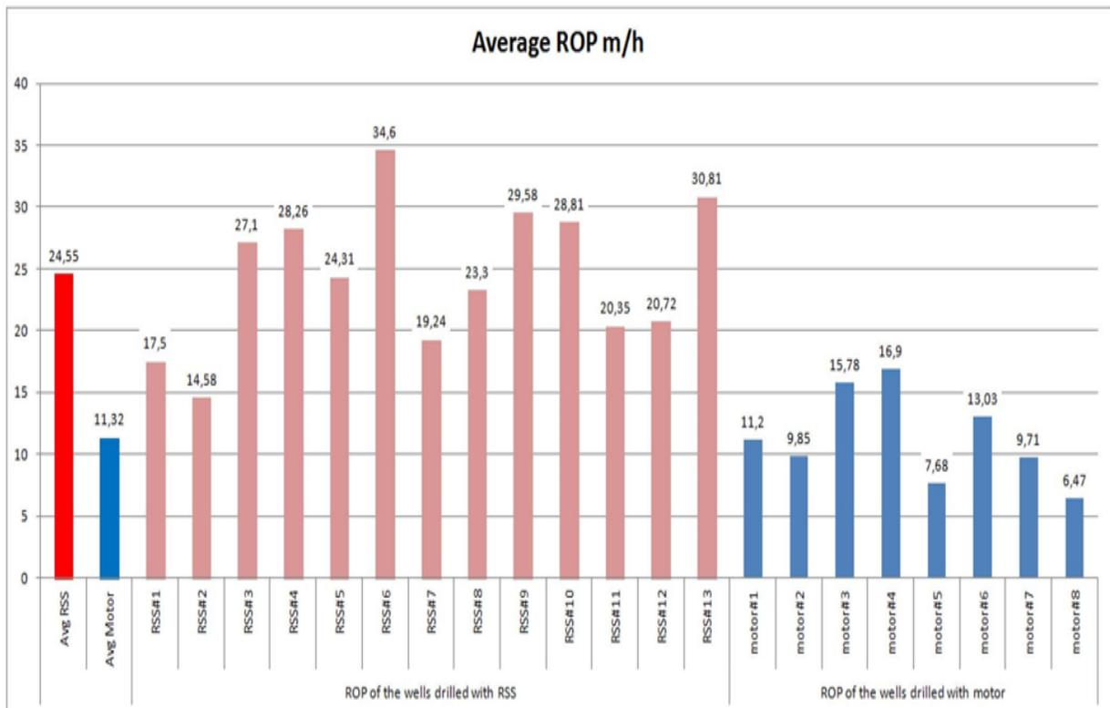
Figure 5-4 ROPs with RSS and mud motor(Wiktorski et al., 2017)
