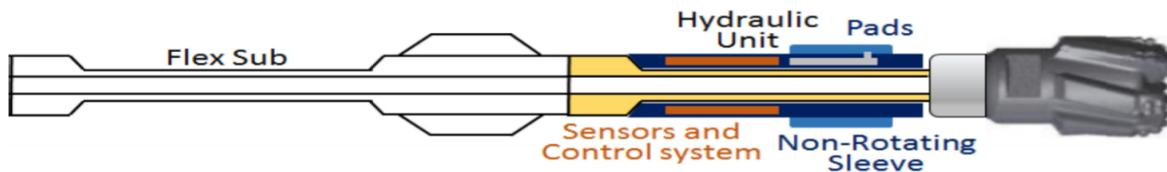
Figure 4-7 Push-the-bit RSS with non-rotating sleeve (Thaiprasert et al., 2016)
