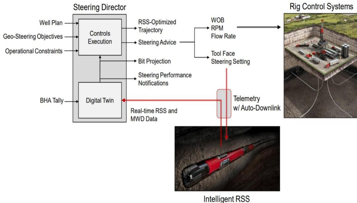
Figure 4-11 Overview of steering advisory and control process(Zalluhoglu et al., 2019)
