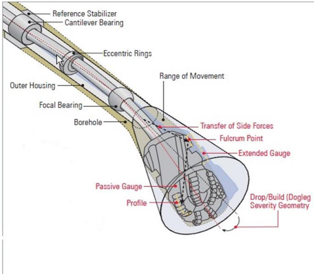
*Figure 4-15 Geo-Pilot Rotary Steering Drilling Tool Working Principle (Portillo et al., 2011)*
