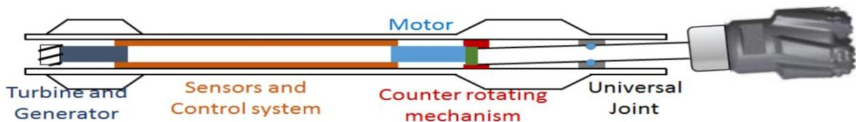
Figure 4-3 Fully-rotating Point-the-bit RSS (Thaiprasert et al., 2016)
