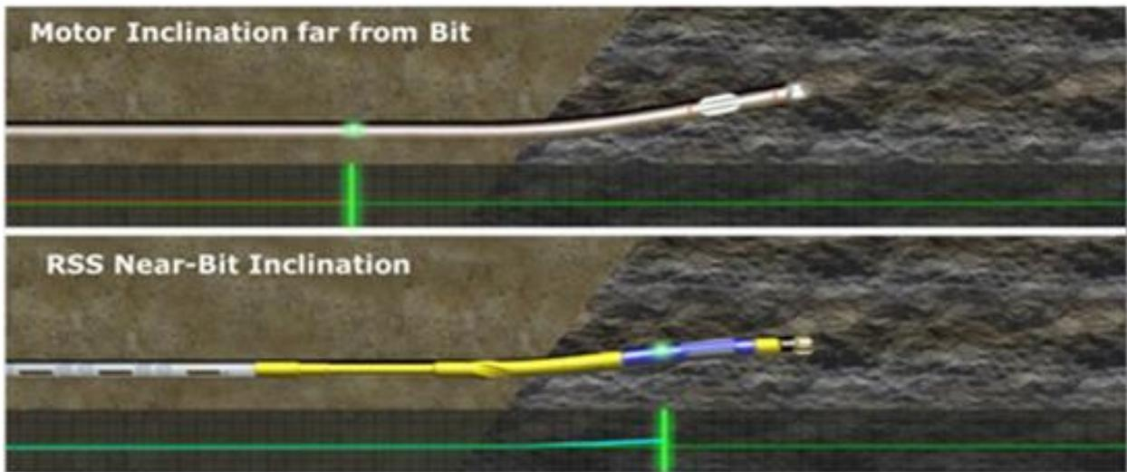
*Figure 4-1 Inclination from bit (Dabyah et al., 2016)*
