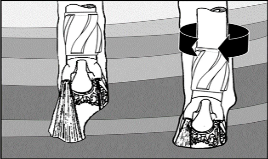
Figure 2-2 Jetting and drilling action (INTEQ & Drilling, 1995)
