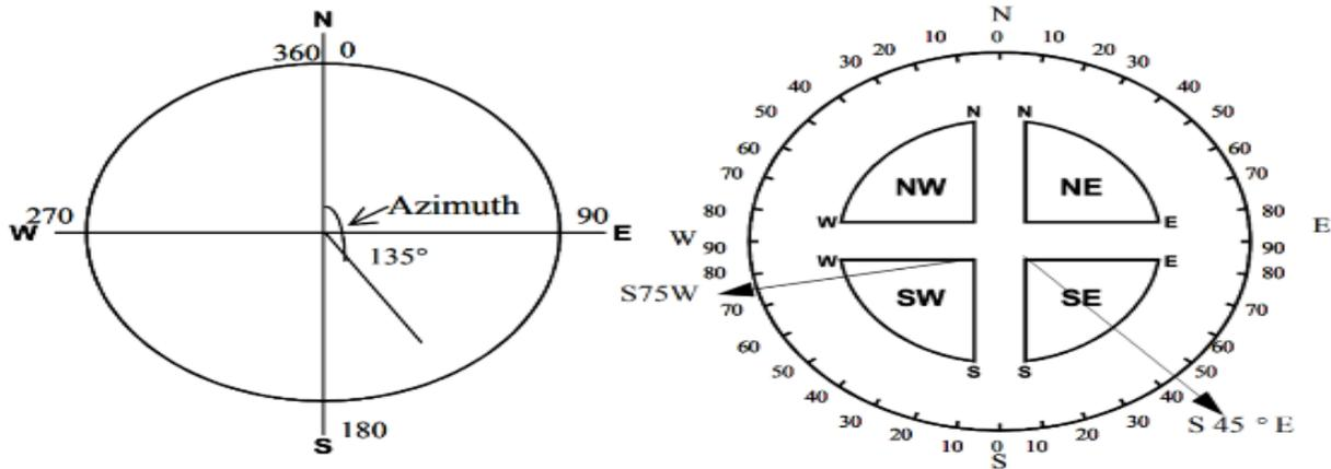
*Figure 1-3 definition of azimuth (Rabia, 2002)*
