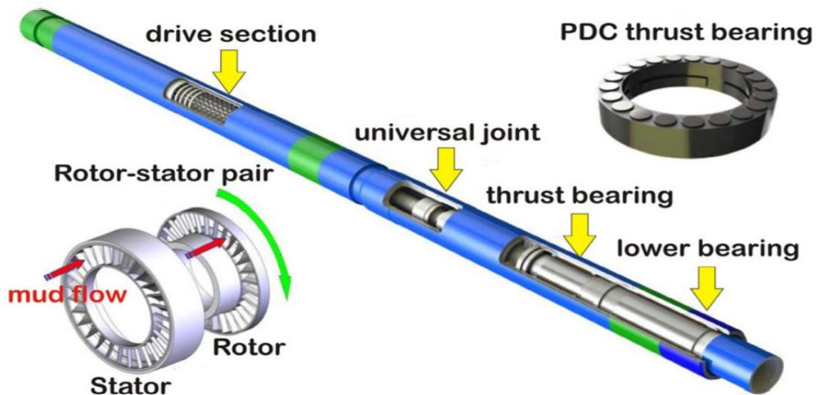
Figure 3-2 Turbodrill Motor (Ma et al., 2016)
