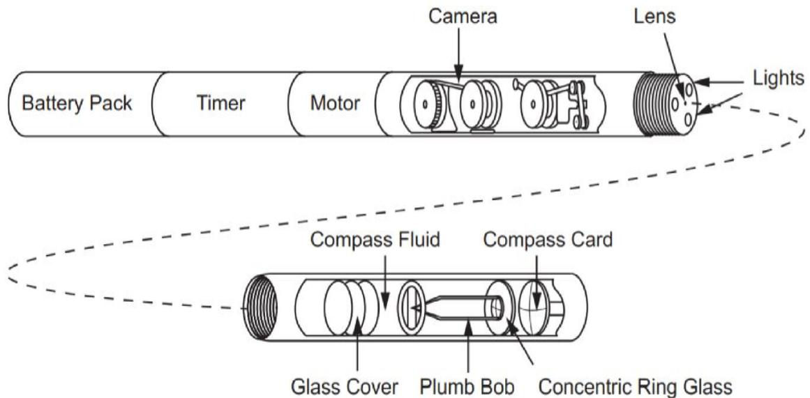
*Figure 2-13 Magnetic Multi shot Device (HERIOT WATT UNIVERSITY, 2005)*
