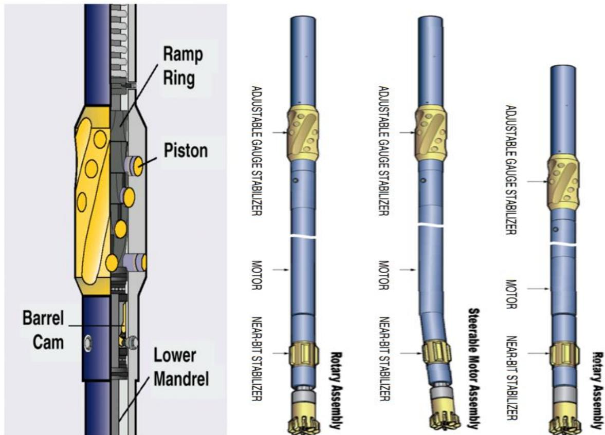
Figure 3-4 AGS with reduced gauge and full gauge (Lawrence et al., 2001)
