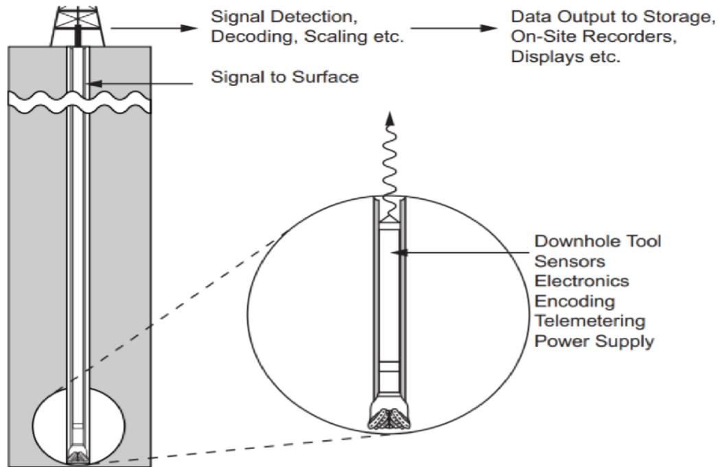
Figure 2-14 Telemetry Surveying Techni (HERIOT WATT UNIVERSITY, 2005)
