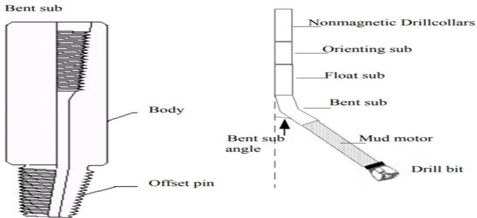
Figure 2-4 PDM BHA with bent sub (Rabia, 2002)
