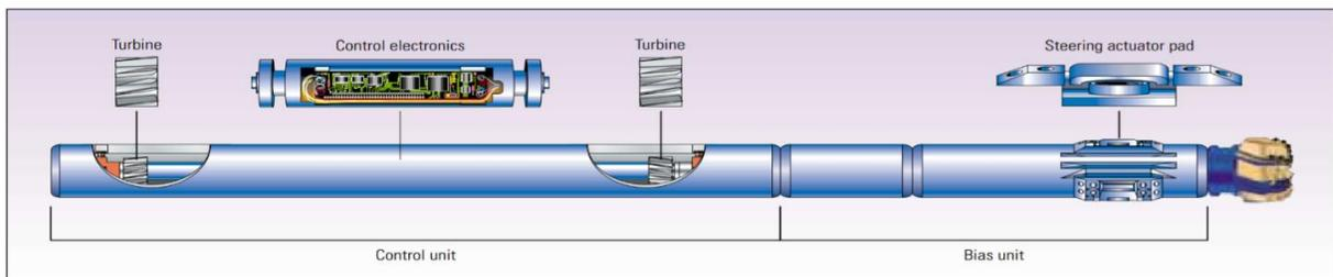
*Figure 4-17 The PowerDrive rotary steerable system (Underdown, 2000)*
