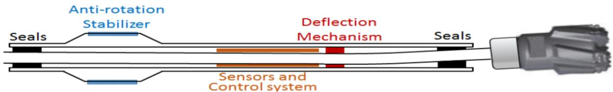
Figure 4-2 Point-the-bit RSS with non-rotating collar
