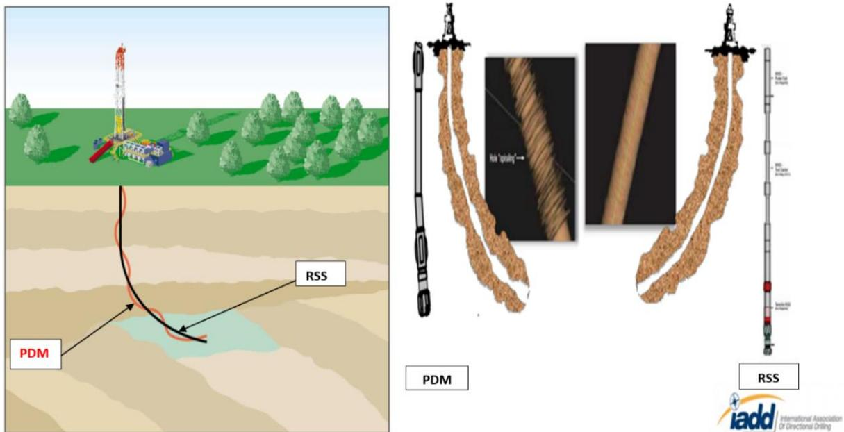
Figure 5-2 PDM vs RSS well trajectory and Tortuosity (adopted from (Lllerhaus, 2019)& (Geoff Downton, 2000)
