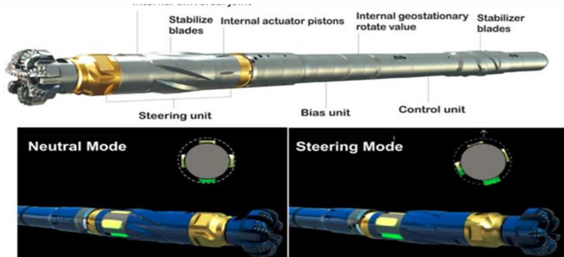
*Figure 4-18 the Schlumberger Power Drive Archer system (Underdown, 2000)*
