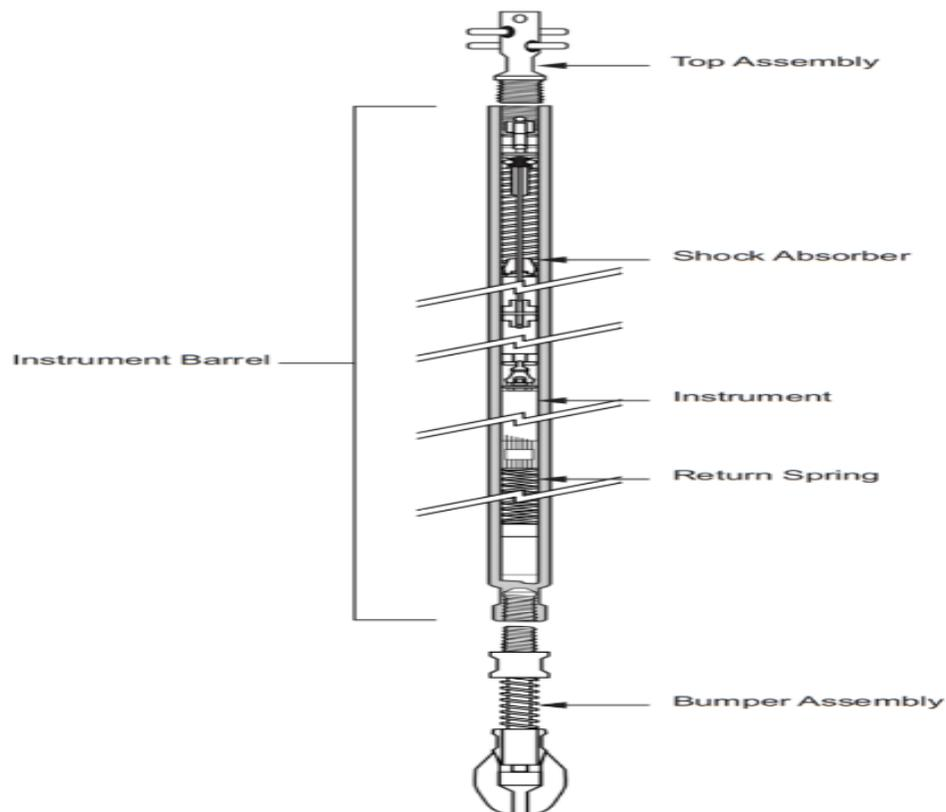
Figure 2-12 Magnetic Single Shot Device (HERIOT WATT UNIVERSITY, 2005)
