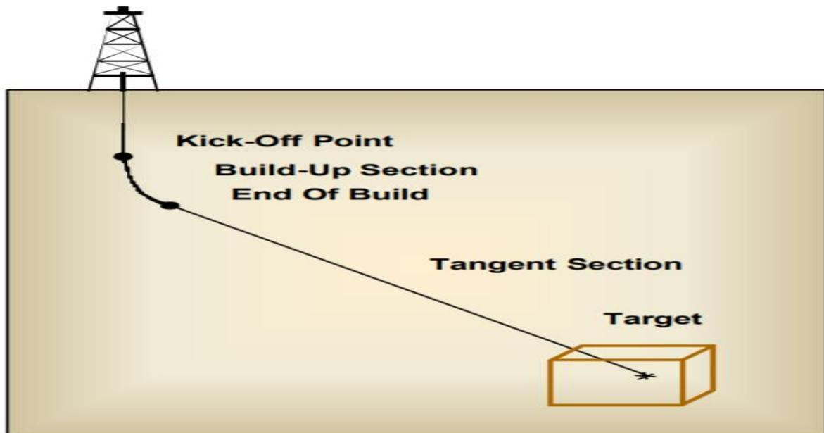
Figure 1-6 Build and Hold (INTEQ, 1996)
