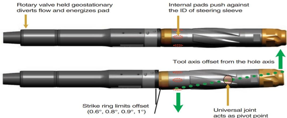
Figure 4-9 the RSS incorporating developed "push-the-bit and point-the-bit" RSS technology (Schlumberger, 2013)
