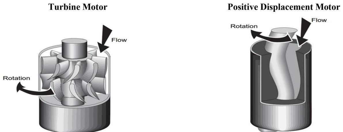
*Figure 3-1 Principles of operation of turbine and PDM (Schlumberger, 1996)*
