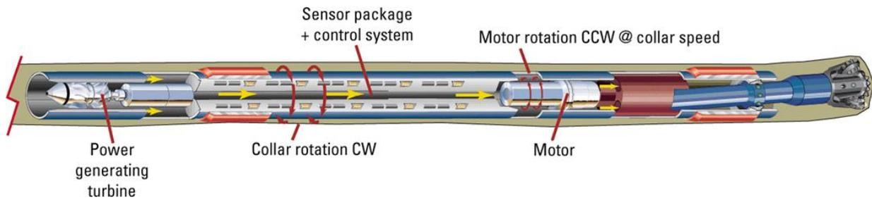
Figure 4-4 Point the bit system in bent mode (Schaaf et al., 2000)
