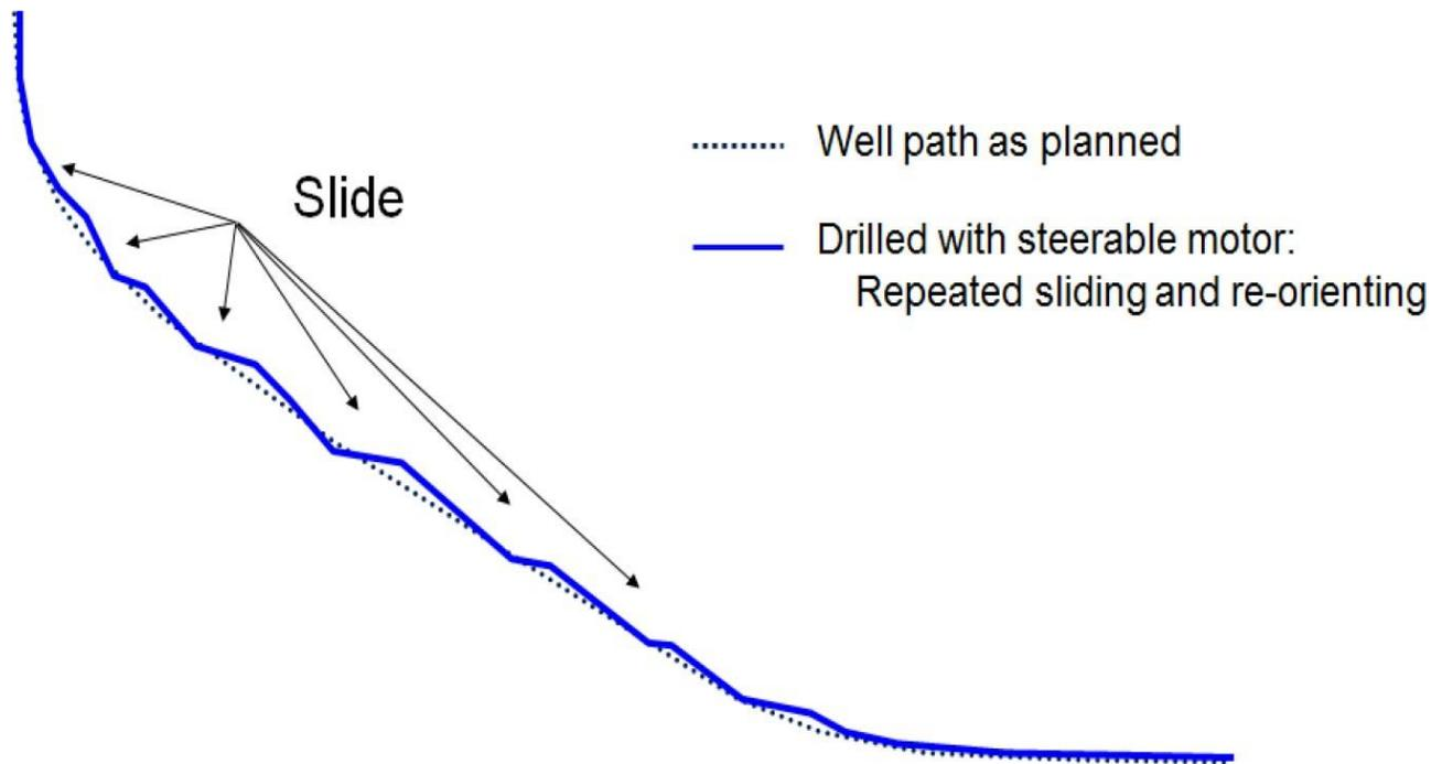
*Figure 3-6 MTR Drilling Modes (Dabyah et al., 2016)*
