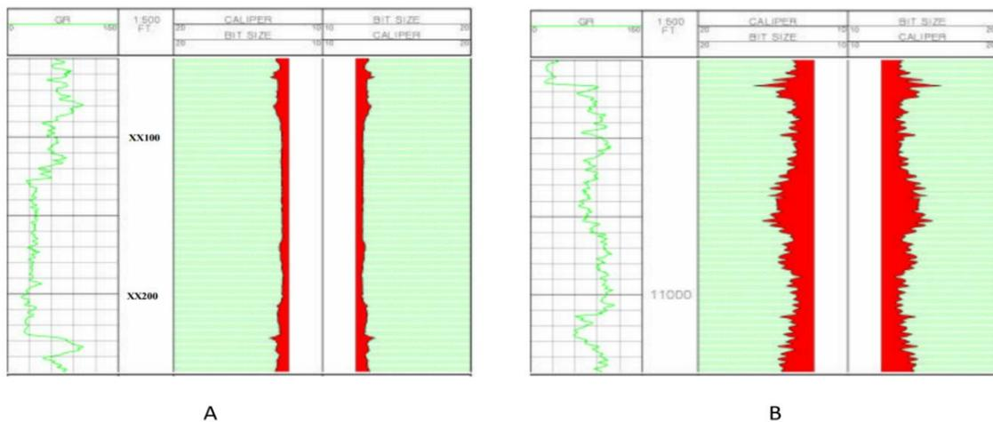
Figure 5-1 (A. Geometry of Borehole Using RSS,B. Borehole Geometry Using Steerable Motor Conventional)( Adopted from (Moody et al., 2005) )
