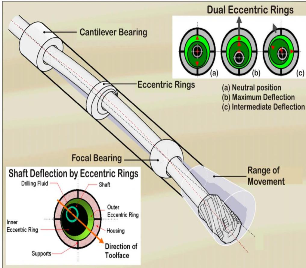
Figure 4-16 Eccentric rings (Ma et al., 2016)
