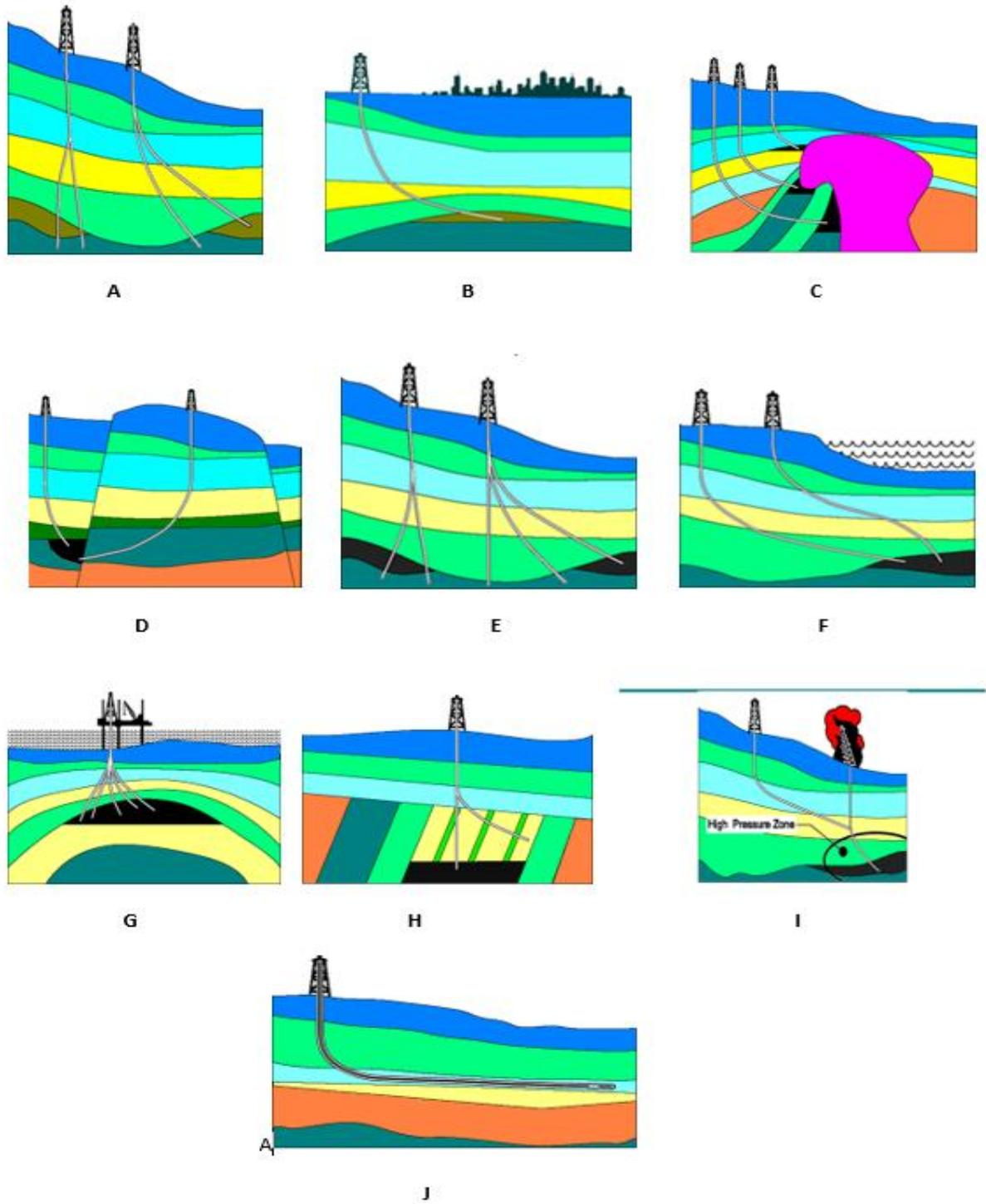
Figure 1-9 directional drilling application (Schlumberger, 1996)
