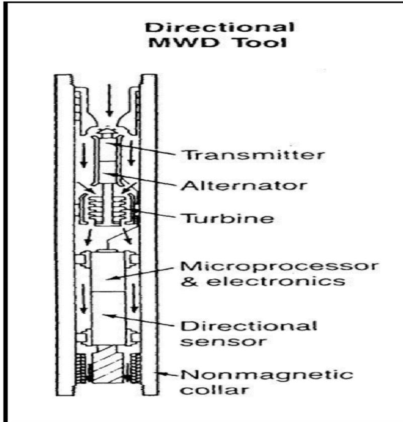
*Figure 2-15 Simplified Diagram of MWD (Carden & Grace, 2007)*
