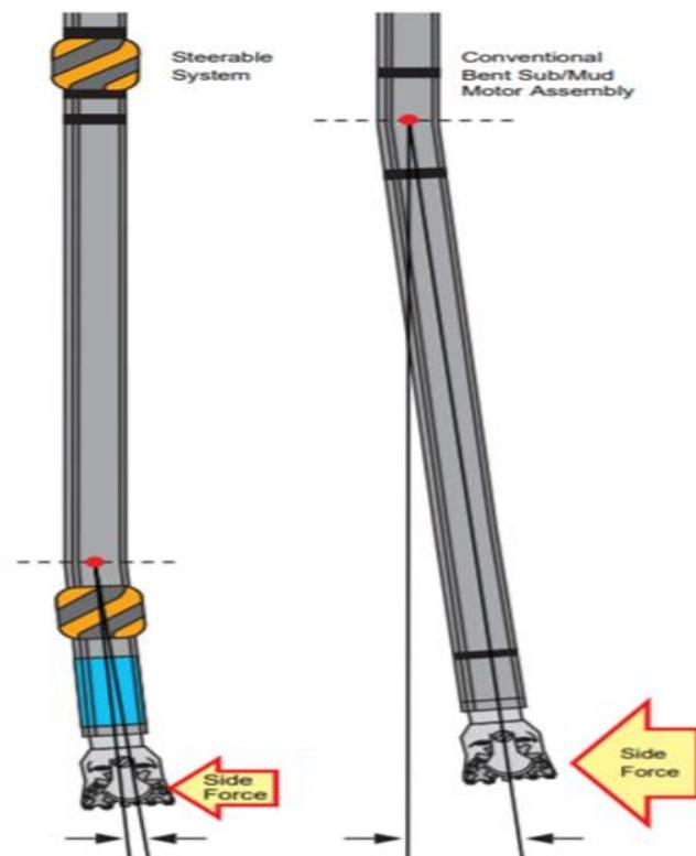
Figure 2-6 Steerable motor bit offset (Schlumberger, 1996)
