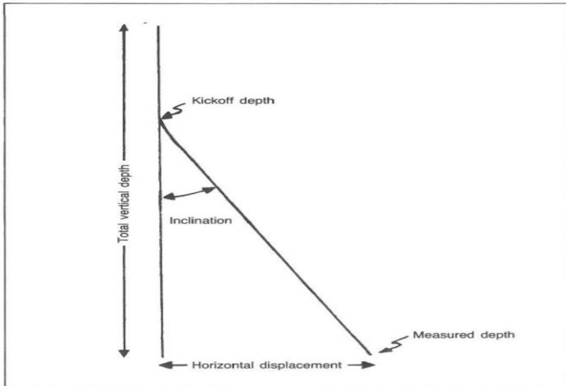
*Figure 1-2 aspects for directional plan drilling(Charrier, 1985)*
