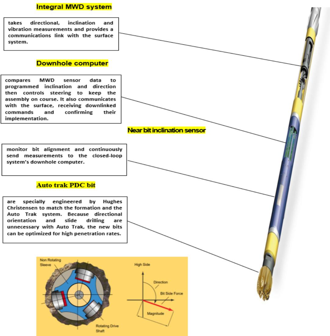
Figure 4-14 Advanced downhole system (HUGHES, 1999)
