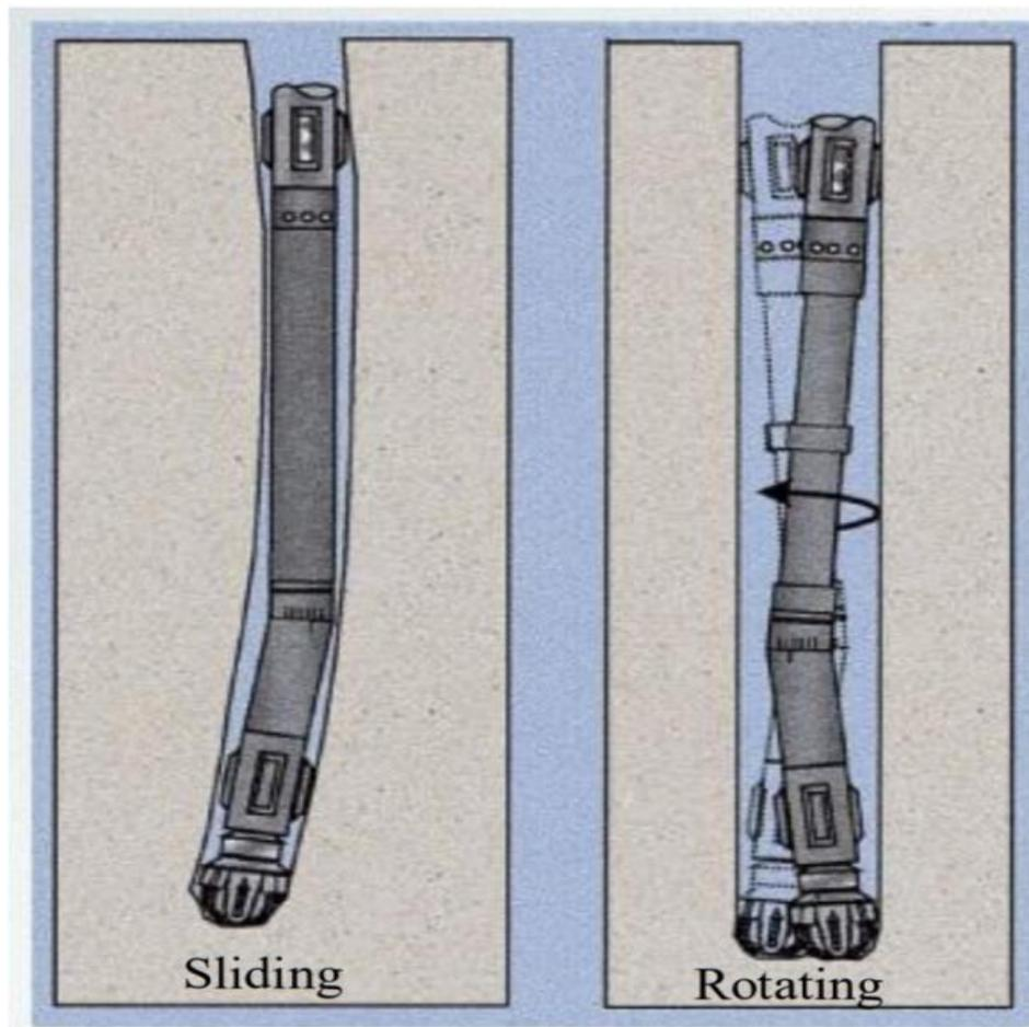
Figure 3-8 Sliding vs Rotating (Warren, 2006)
