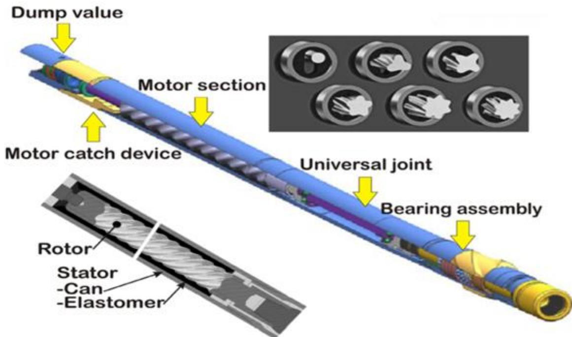
Figure 3-3 the schematic diagram of a typical PDM tool (Ma et al., 2016)
