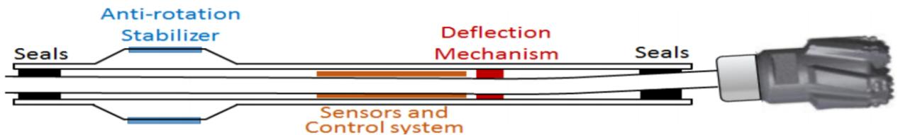
Figure 4-2 Point-the-bit RSS with non-rotating collar
