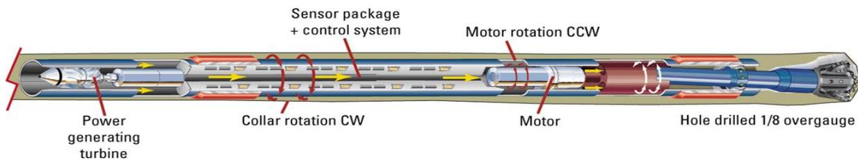
Figure 4-5 Point the bit tool in the straight mode; it is permitted to nut the bit shaft, leading in a hole slightly and over gauge (Schaaf et al., 2000)
