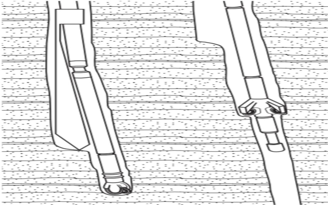
*Figure 2-1 Whip stock operation (HERIOT WATT UNIVERSITY, 2005)*
