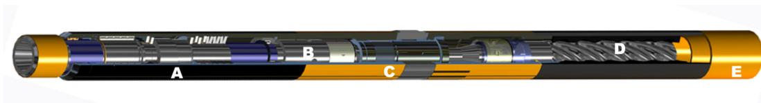
Figure 2.18: (A) Bearing Assembly, (B) Universal Joint Assembly, (C) Adjustable Bent Housing/Fixed Housing, (D) Power Sections, (E) Dump Valve/Blank Sub
