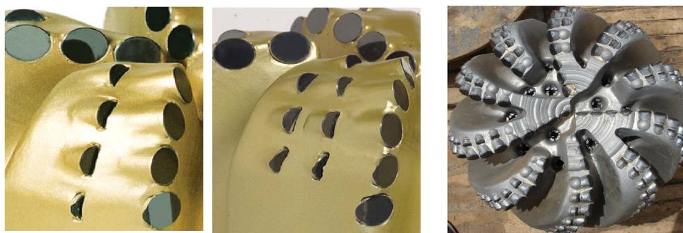
**Figure 4.9:** Backup cutters(L), PDC design with 10 blades,19-mm cutters achieved the fastest ROP(B), [15].
