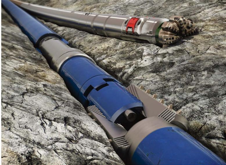
**Figure 2.14:** Sidetracking after pumping cement. With its anchor in place, the Track-Master OH-C system permits drillers to sidetrack without having to wait for cement to cure,[10].
