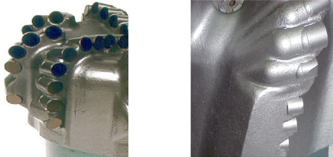
**Figure 4.4:** PDC bit with active gage configuration(L) and PDC bit with reduced side-cutter count(R), [40].
