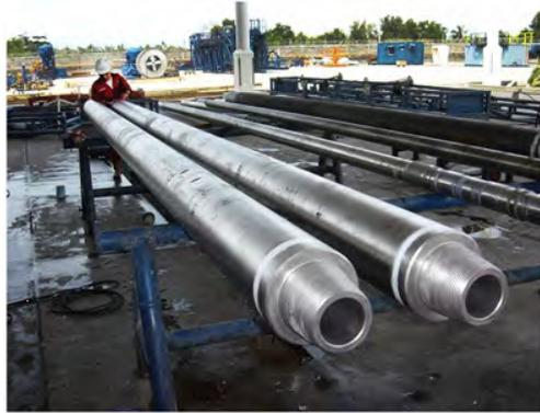
**Figure 3.4:** A non-magnetic drill collar (NMDC), [27].
