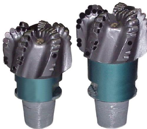
**Figure 4.5:** Difference in Make up Length
