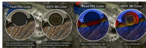
**Figure 4.7:** The comparison of fixed PDC cutter and ONYX 360 cutter
