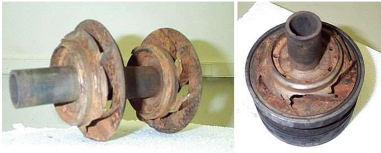
Figure 18: Impeller damage due to thrust
