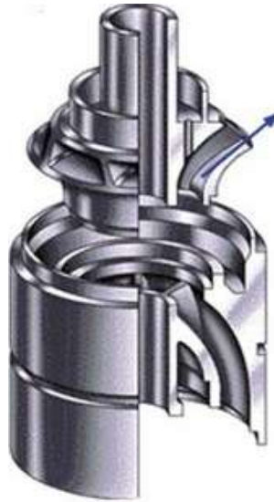
Figure 17: Mixed flow stage
