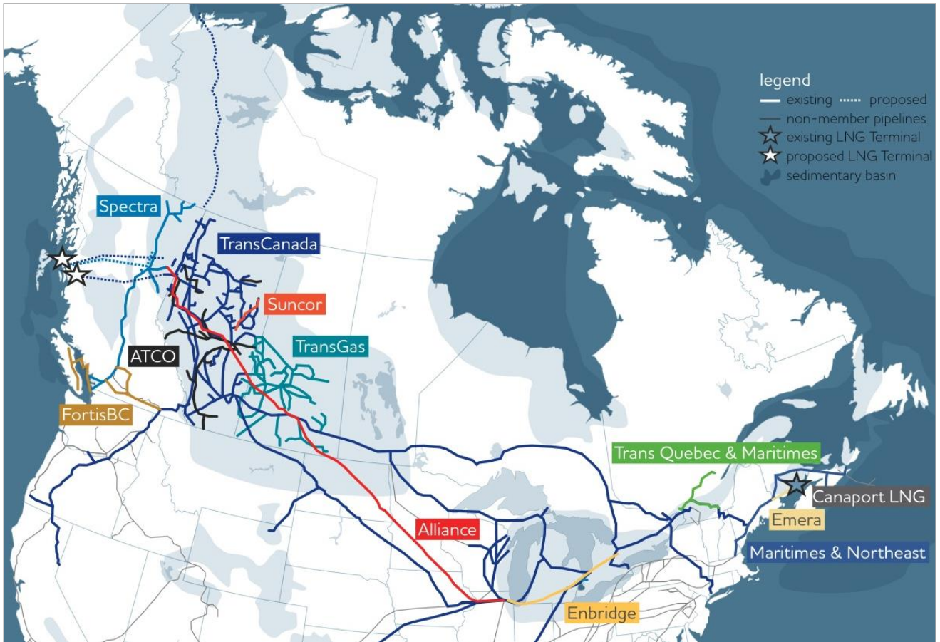
Figure 16 CEPA members' natural gas transmission grid [21]
