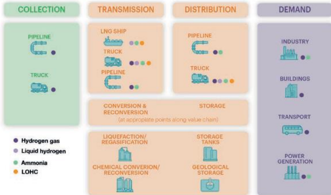
Figure 5 Possible forms and means for hydrogen transportation at different levels of the supply chain, [2]
