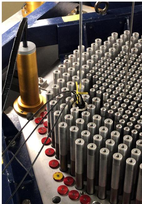
**Figure 3.1:** Picture of the CROCUS core with the experimental instrumentation inserted in the NW control tube for the testing of the detection system.
