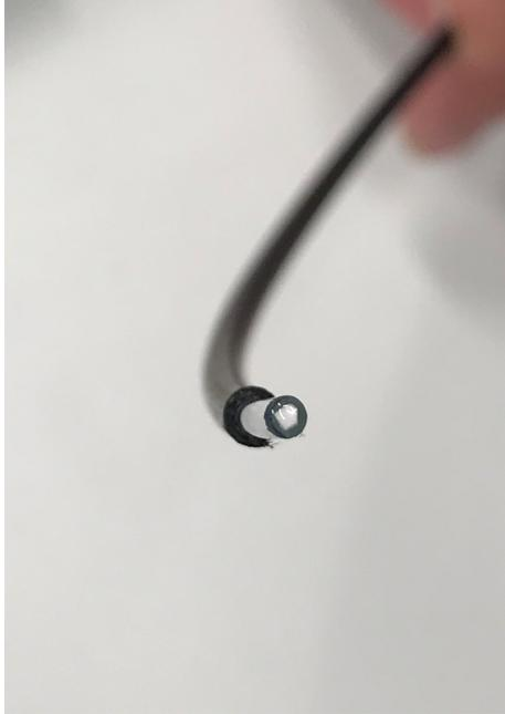
**Figure 1.13:** Picture of the miniature fiber detector. As the protective Aluminum cap is removed, the scintillator screen is visible (in white).
