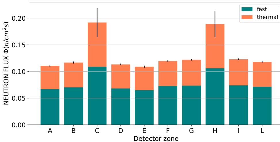
**Figure A.3:** Neutron flux distribution around the reactor concrete shielding.
