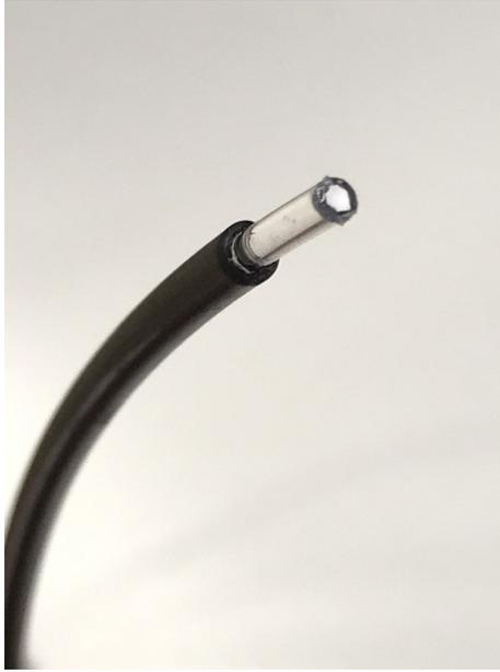
**Figure 3.2:** Picture of the front-end of the detector. The scintillator is visible as the aluminum cap is here removed.
