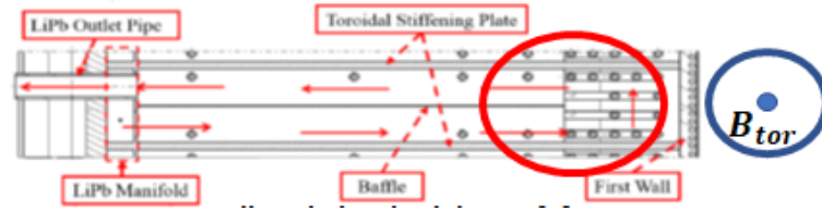
Figure 4.11: BZ cell: radial-poloidal view. The U-turn is highlighted in the red circle and the toroidal magnetic field is indicated by a blue arrow (perpendicular to the figure) [32].
