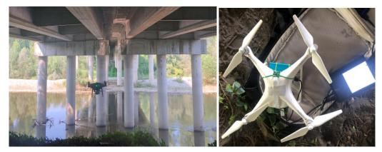
Figure 44. Modified drone during the survey activity.
