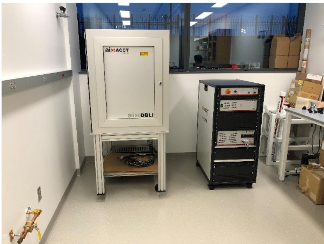
**Figure 3.9:** Picture of the AixDBLI tool. On the right, the case, amplifier and system to suppress vibrations. The DBLI is on the left, together with the chuck, onto which wafers or single chips are placed to be tested.
