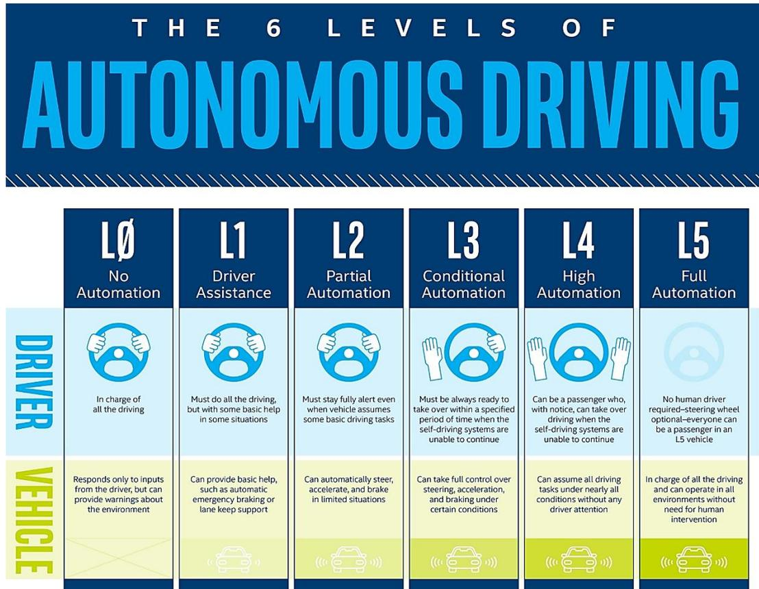
Figure 3.3 The 6 levels of autonomous driving – Society of Automotive Engineers (SAE); National Highway and Traffic Safety Administration (NHTSA) – INTEL
