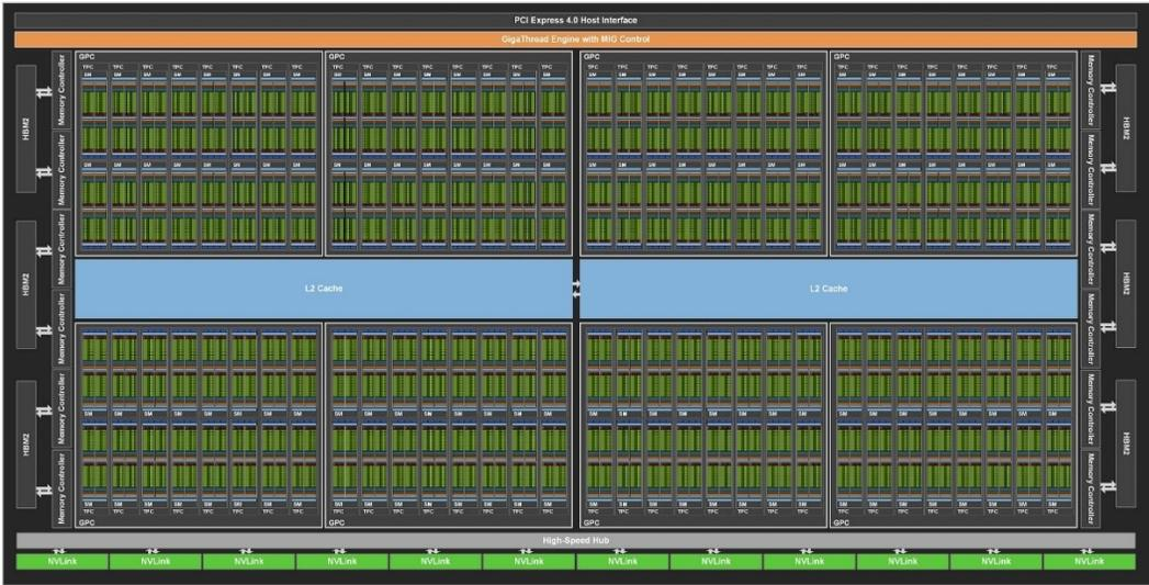
Figure 2-19 Nvidia GA100 Top-level Architecture, [30]
