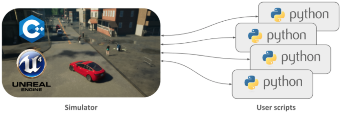
Figure 3: Server-Client communication through Python API.
