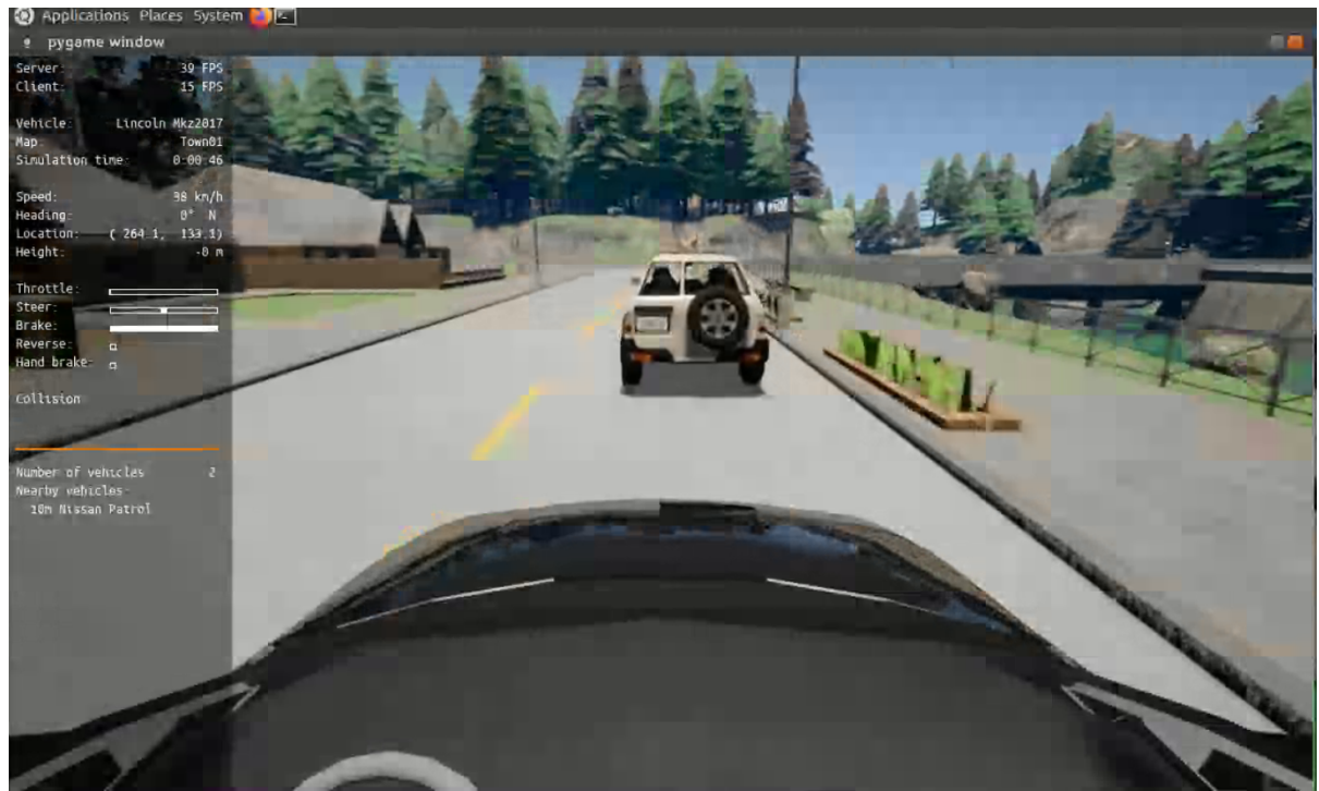
Figure 4: Interface with the pygame window. It is evident how on the left there are a lot useful information such as: throttle value, brake value, steering angle, distance from the leading vehicle, etc.
