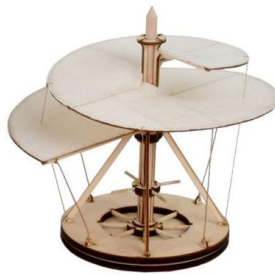
Figure 1.1: "aerial screw" prototype as designed by Leonardo da Vinci [1]
