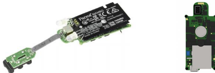
Figure 4.5: motherboard of Mambo fly model [27]
