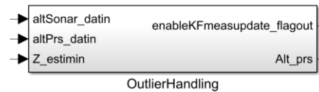
Figure 6.49: Outlier Handling subsystem block (part of the Altitude estimator)
