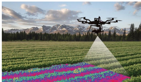
Figure 1.4: Airborne Hyperspectral sensor [6]
