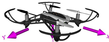
Figure 5.19: reference frame of Quadcopter model [31]
