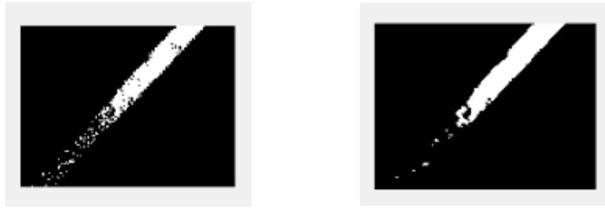
Figure 9.3: Issue related to wrong filtering of the track due to darker regions of the path
