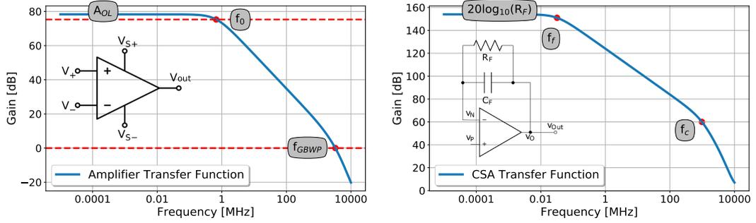
**Figure 2.5:** The amplifier frequency response shows essential information for the CSA design optimization.  $f_{GBWP}$  frequency is defined at unity-gain (0 dB), and relates to how fast the amplifier responds [left]. The integration behavior of the CSA topology [right] lasts from  $f_f$  to  $f_c$  frequency range.
