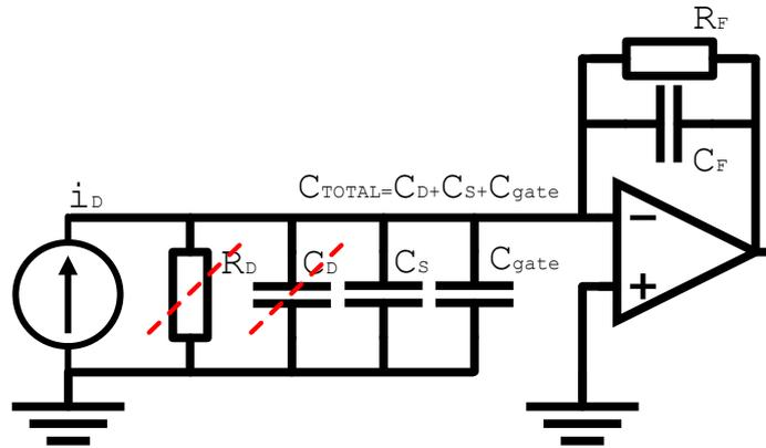
**Figure 2.3:** Front-end readout circuit of a charge-sensitive amplifier. Equivalent sensor circuit couples to the CSA configuration.  $C_D$  is in the order of a few fF compared to  $C_{gate}$  and  $C_S$  in the pF range;  $R_D$  is in the order of G $\Omega$ , much higher than the OPA impedance. Both elements can be disregarded.
