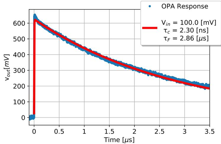
**Figure 3.4:** Charge Sensitive Amplifier signal response to a rectangular pulse; small overshoot occurs because the passive probe loads the output.
