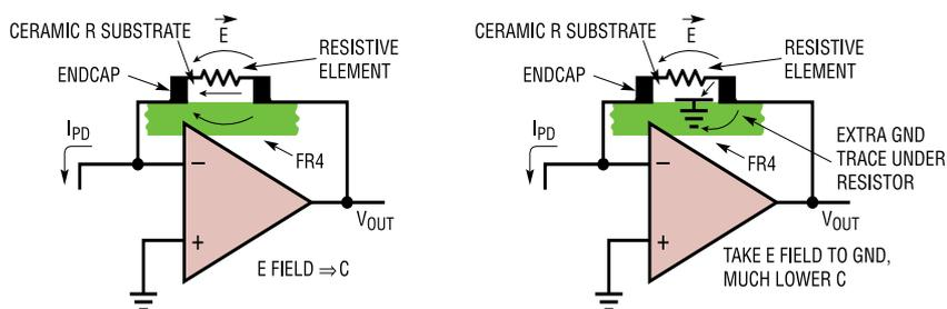
**Figure 6.1:** Normal layout (left) and Field-Shunting layout (right); minimal pad sizing and enhanced layout reduces *Miller capacitance*, extending bandwidth and improving noise performance. Adapted from [32]
