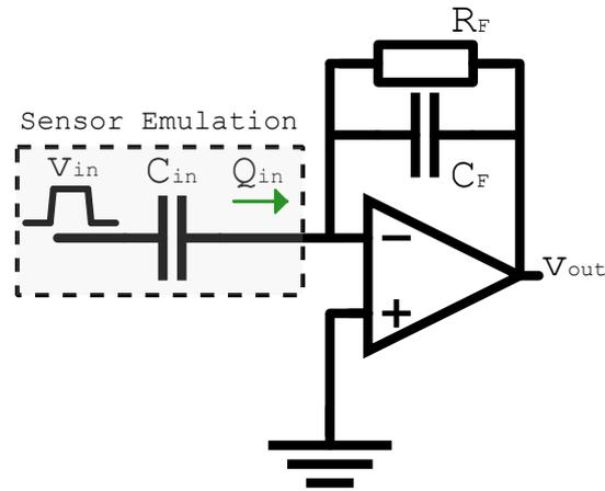
**Figure 3.2:** Pulser circuit. When driven by a voltage waveform source  $V_{in}$ , the capacitor  $C_{in}$  provides an equivalent charge  $Q_{in}$ .
