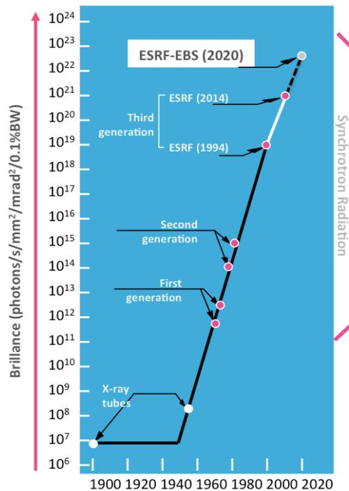
**Figure 1.2:** Since the 1950s, X-ray source brilliance has increased orders of magnitude over the years, dictating synchrotron family generations. Adapted from [9].
