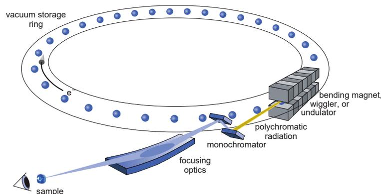
**Figure 1.1:** Schematic view of a synchrotron light source. Storage rings are powerful X-rays sources designed and dedicated to generate tunable photon beams from the far-infrared to the hard X-ray regime (1 meV - 150 keV). Adapted from [3].
