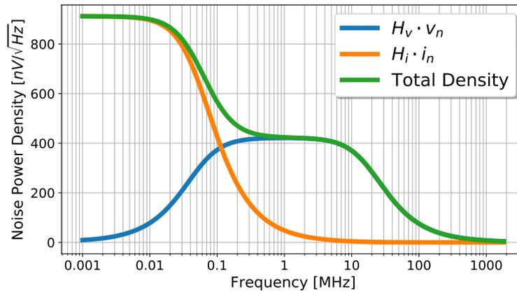
**Figure 2.13:** Noise spectral density plot for the charge-sensitive amplifier. The frequency response of the  $i_n$  has the shape of a low-pass filter; the component related to  $v_n$  has the response of a band-pass filter.
