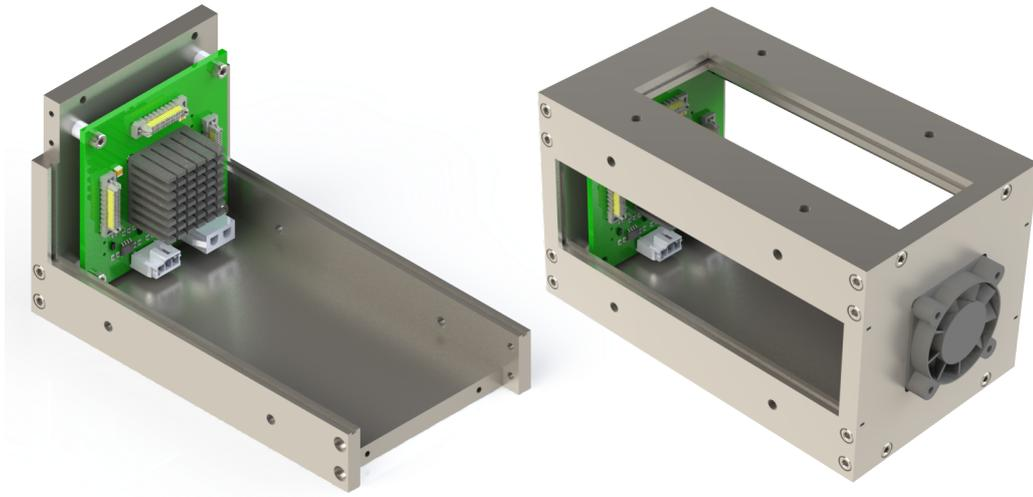
**Figure 4.5:** Power supply components are placed at the bottom of the sensor board; high-speed connectors on the periphery bring the sensor signal to the readout circuit, placed on a distinct PCB. The cooling fan makes turbulent the air inside the case, facilitating heat exchange.
