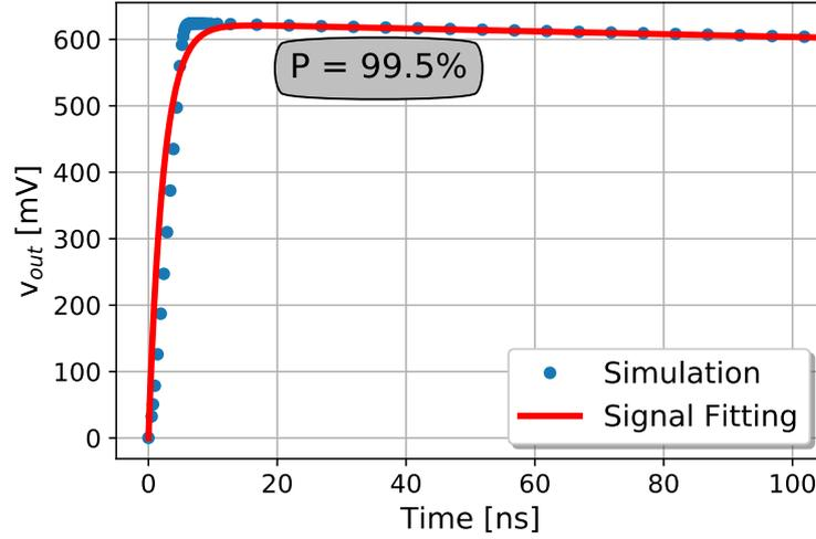
**Figure 3.6:** Effect of the ballistic deficit on the pulse height. A peak amplitude inferior to 2% compared to the theoretical signal is considered appropriate.
