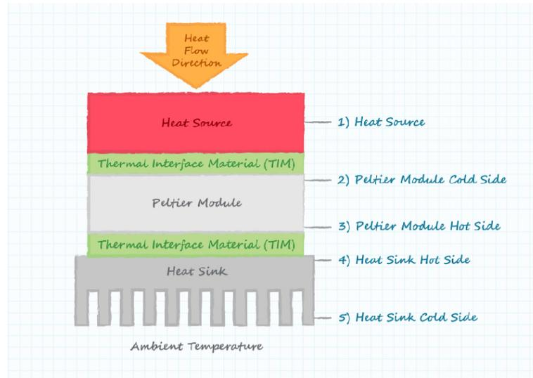
**Figure 4.3:** Peltier power dissipation system. Accurate thermal analysis requires dedicated simulation tools to understand the heat dynamics. Adapted from [36].
