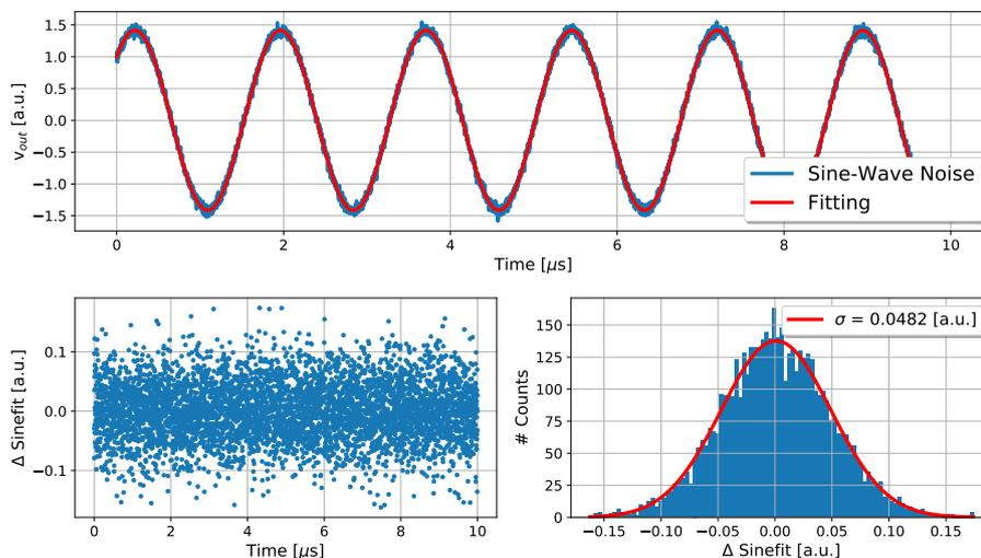
**Figure 3.7:** Example of noise measurement of the charge-sensitive amplifier using the sine-wave method. The noise is superimposed to the output signal [top]. The fitting residuals are presented in the time domain [lower left], while the standard deviation of the histogram plot [lower right] expresses the system noise.
