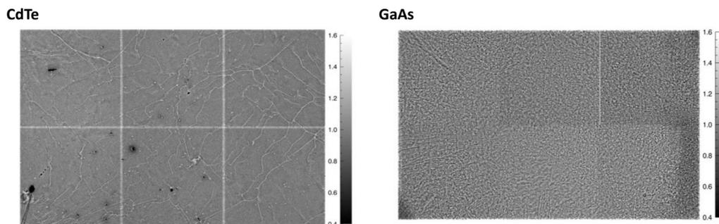
**Figure 1.5:** Flat-field images of high-Z sensors show imperfections, generally not stable over time. Adapted from [16].
