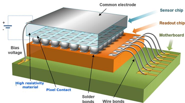
**Figure 1.6:** Generic architecture of a hybrid pixel detector. The pixelated semiconductor sensor is connected to the CMOS readout ASIC by means of bump bonding technology. Adapted from [18].
