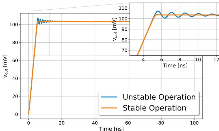
**Figure 2.9:** Circuit stability is a major concern for the CSA implementation. The feedback network can cause distortions and signal overshoots if not properly designed.
