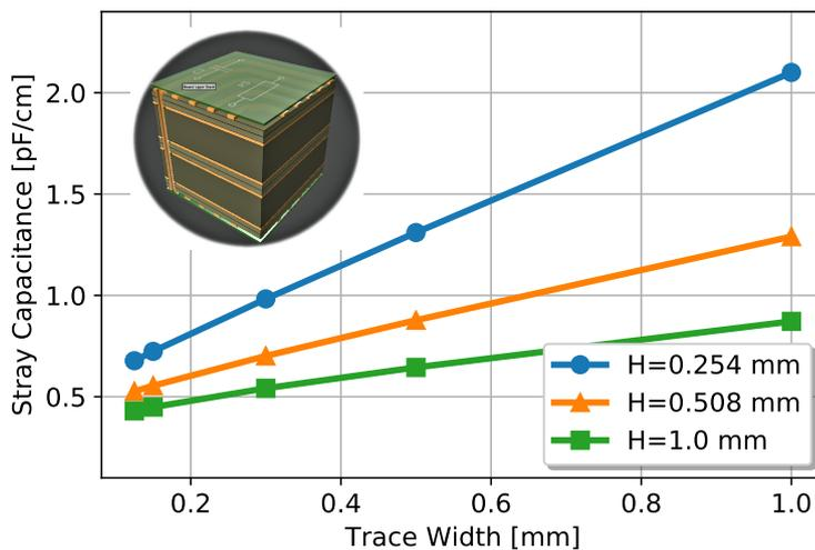
**Figure 4.2:** Separating GND/Power planes away from the signal traces reduce  $C_S$  drastically; trace width shows a minor impact for thin interconnections. Data gathered from Saturn PCB Toolkit [34].
