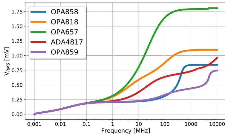
**Figure 2.14:** Converting noise spectral density into RMS noise voltage evidences that the total noise saturates at high frequencies since the CSA does not integrate the signal above the cutoff frequency.
