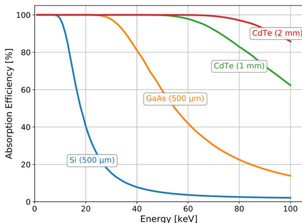
**Figure 1.4:** Comparative absorption efficiency curves for different sensors materials over a wide X-ray energy range [12, 13]. NIST XCOM database [14].
