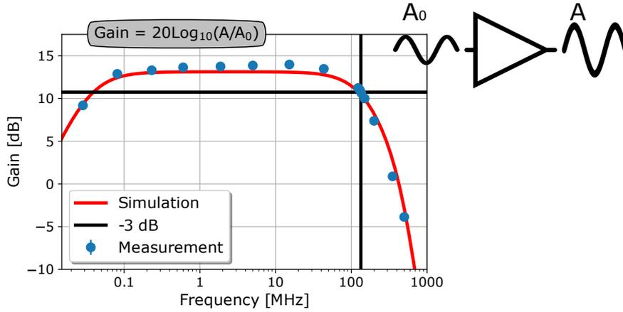
Figure 3.3: Bode diagram plot of the circuit frequency response.
