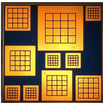
**Figure 4.1:** CdTe prototype chip has total area of  $13 \times 13 \text{ mm}^2$ ; the readout electronics is directly connected to each pixel. Adapted from [25].
