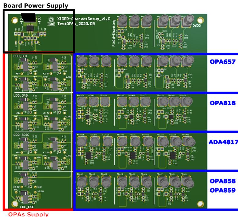
**Figure 3.1:** Characterization PCB used for front-end electronics validation. The testing platform is also used for debugging purposes to identify possible circuit optimizations. Implemented using Altium Designer software.
