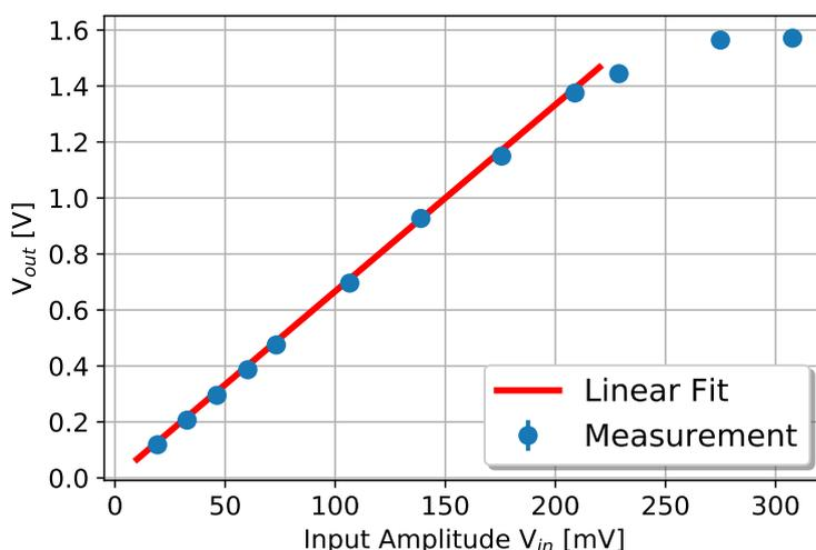
**Figure 3.5:** Variation of the output peak height for an given input amplitude  $V_{in}$ . Signal distortion is observed when the OPA is forced into saturation condition.
