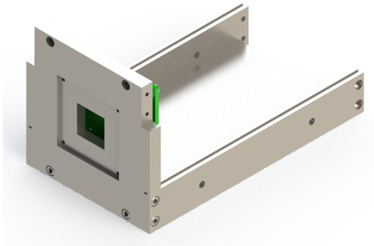
**Figure 4.4:** Assembly of the characterization platform. The sensor is exposed externally through a opening on the front-frame, while the readout electronics remains hidden inside the housing.
