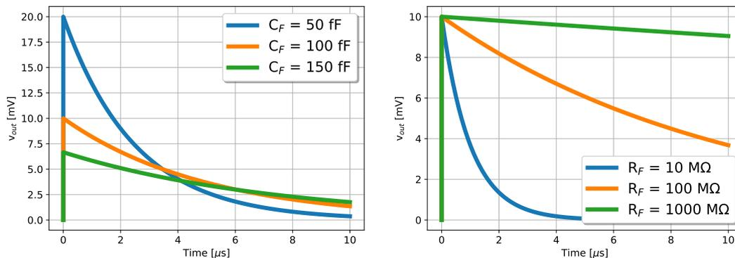
**Figure 2.4:** CSA dependencies for an ideal amplifier in response to a delta-pulse input.
