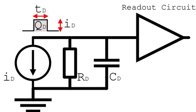
**Figure 2.1:** Equivalent electrical circuit of an X-ray sensor. The characteristics of the sensor influences the behavior of the readout circuit, directly connected to the sensor electrode [19].
