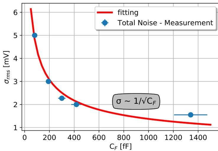
**Figure 3.9:** Simplified fitting model illustrates the noise level respecting the  $1/\sqrt{C_F}$  trend.  $C_{in}$  assumed to be 400 fF.
