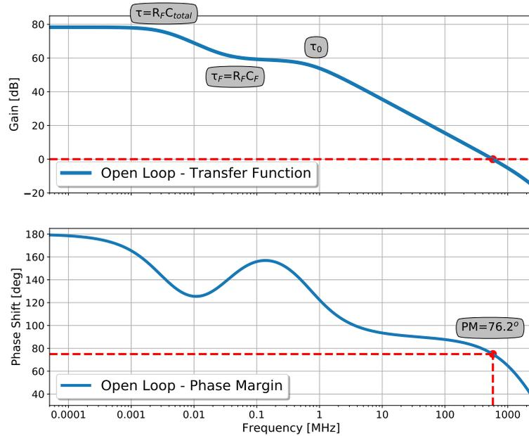
**Figure 2.11:** Open-loop transfer function. At loop gain equals to 1 [top], the phase margin is roughly 76° [bottom]. This is sufficient for a stable operation.
