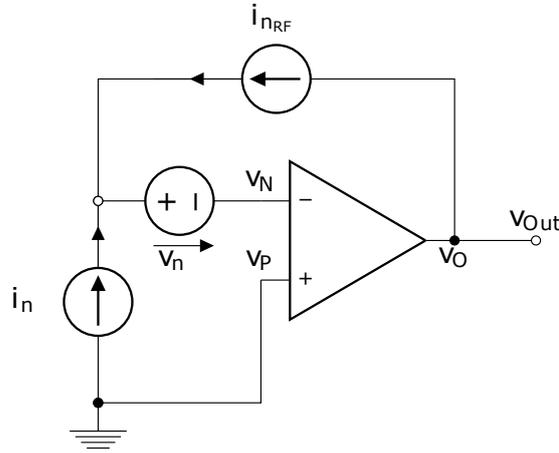
**Figure 2.12:** The charge-sensitive amplifier configuration with its equivalent noise sources. Adapted from [29].
