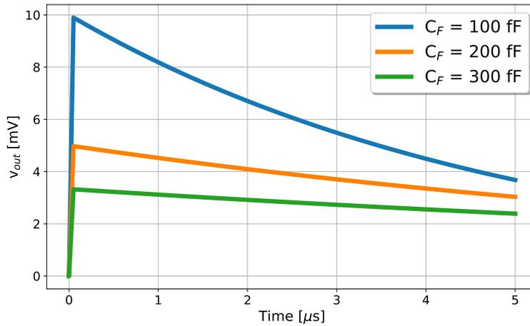
**Figure 2.6:** For a given resistor  $R_F$ , different  $C_F$  leads to different charge-to-voltage gain and discharge profiles, and need to be optimized. The response of the CSA topology to a delta-like pulse is composed of a fast rise-edge component related to the cutoff frequency, and a slow discharge dominated by  $\tau_F$ .
