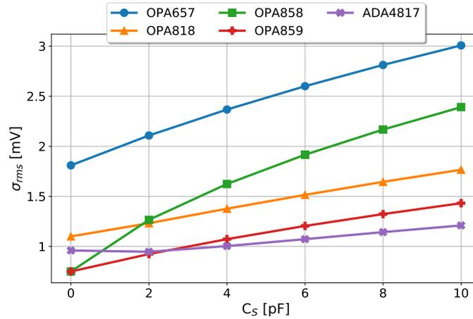
**Figure 2.17:** TINA simulation of the total CSA noise. Large bandwidth amplifiers are more severely impacted by  $C_s$ .
