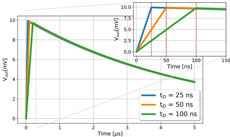
**Figure 2.7:** CSA response to a rectangular current pulse. For a given charge  $Q_D$ , the maximum voltage is reached when the full charge is collected, at the end of the carrier drift time  $t_D$ .
