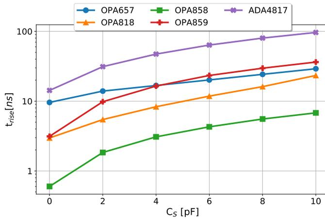
Figure 2.15: Influence of  $C_S$  represents a limiting factor in terms of system rise and bandwidth.
