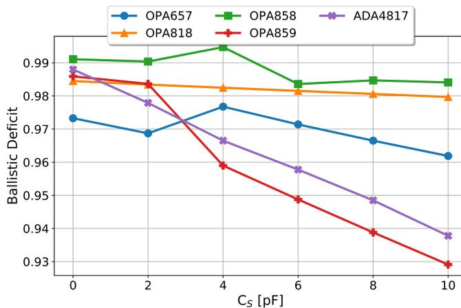
Figure 2.16: Influence of  $C_S$  on the ballistic deficit.  $C_{total}$  slows down the amplifier response, causing some OPAs to be discarded due to their insufficient response
