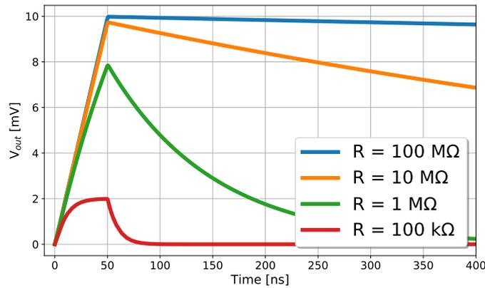
**Figure 2.8:** The ballistic deficit express the loss of output signal amplitude with respect ideal implementation. The maximum voltage is reached when the full charge is collected at the end of the drift time  $t_D=50$  ns.
