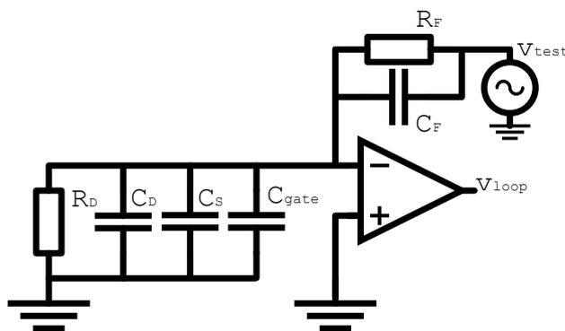
**Figure 2.10:** Open-Loop test circuit. This approach permits to measure the gain given by the feedback components, despite locating key frequencies for the CSA stability analysis.
