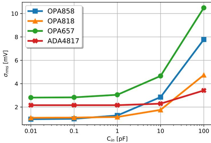
**Figure 3.8:** Dependence of the output noise level with respect to the input capacitance  $C_{in}$ .  $C_F$  assumed constant equal to 100 fF.
