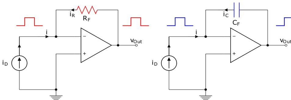
**Figure 2.2:** The TIA [left] is used as a current-to-voltage converter, whereas the CSA [right] is used for a charge-to-voltage conversion.
