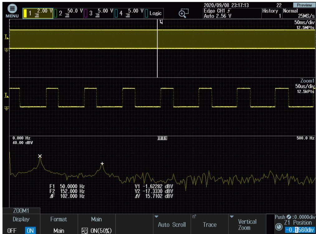
**Figure 4.16:** Spectrum analysis of the PWM signals when the duty cycles are set by the V/f control algorithm.
