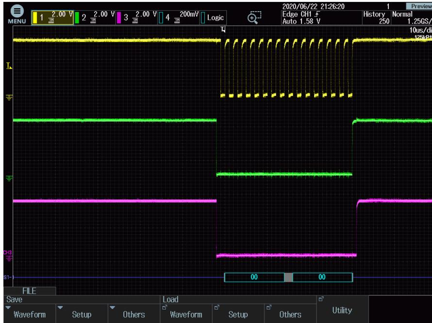
**Figure 4.23:** SPI frame sent by the MCU to configure the R2D converter at startup.
