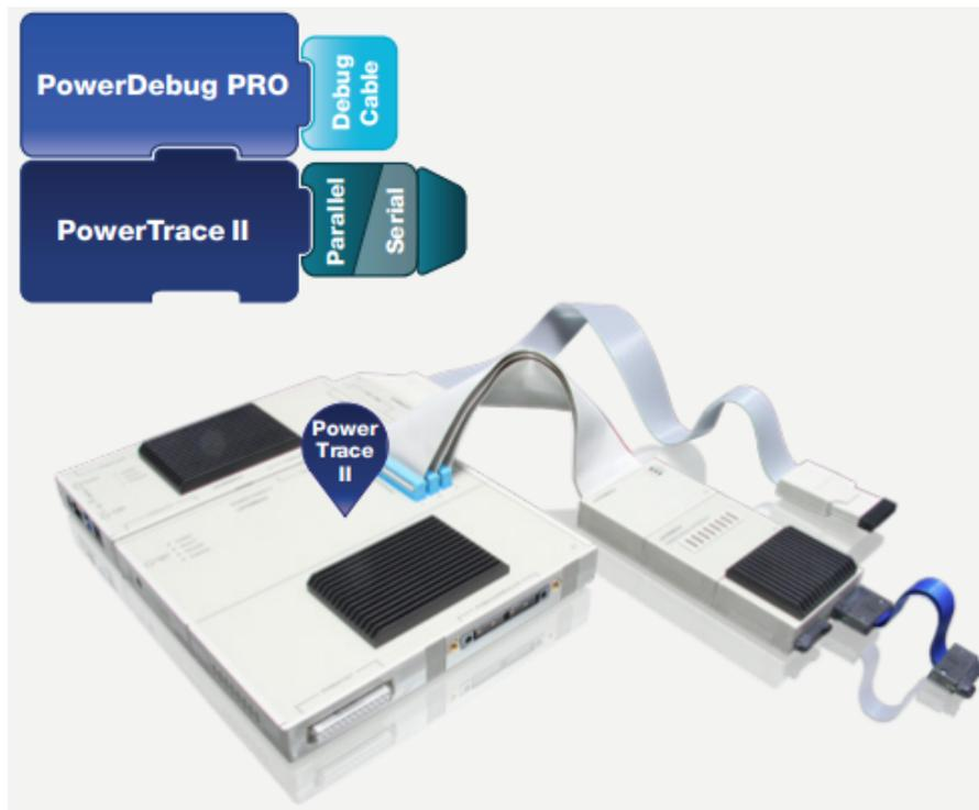
**Figure 4.4:** Lauterbach Debug and Trace hardware tools structure used for firmware testing [7].
