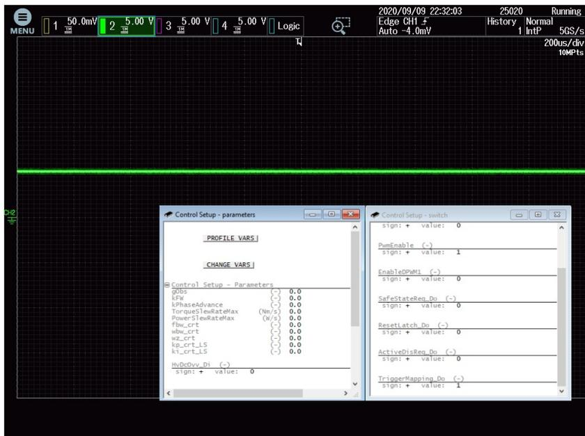
Figure 4.27: Screenshot of the acquisition of the digital input signal when the corresponding voltage level is set to 1.
