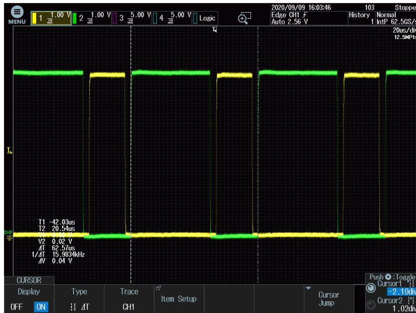
**Figure 4.13:** Screenshot of the acquisition of two PWM complementary signals with switching period measurement.
