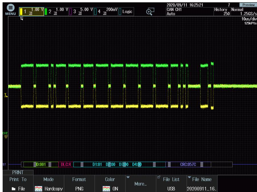
**Figure 4.35:** Screenshot of the acquisition of the TX message 02 sent by the MCU node.
