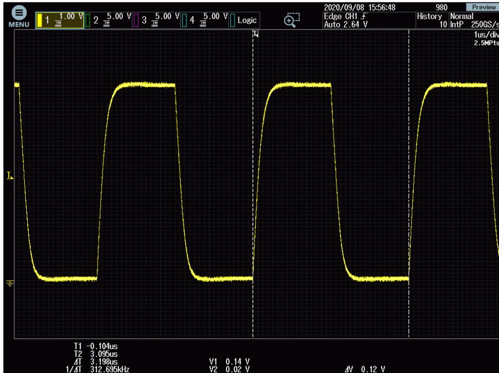
**Figure 4.11:** Frequency measurement of the MCU clock signal HSE\_IPG\_CLK.
