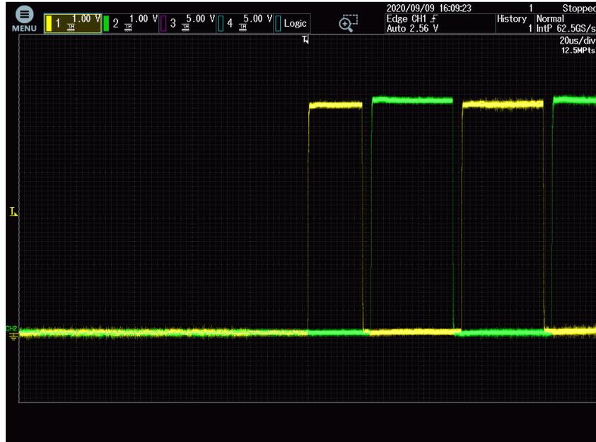
**Figure 4.15:** Screenshot of the acquisition of the enabling of two PWM complementary signals.
