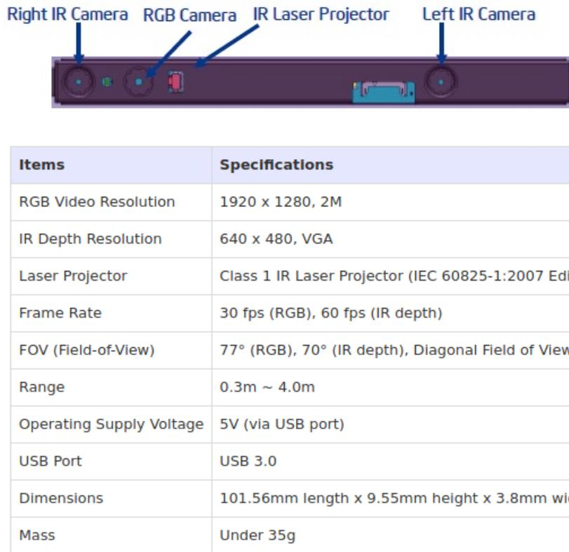
**Figure 5.4:** Intel RealSense R200 labels and technical specification.[28]
