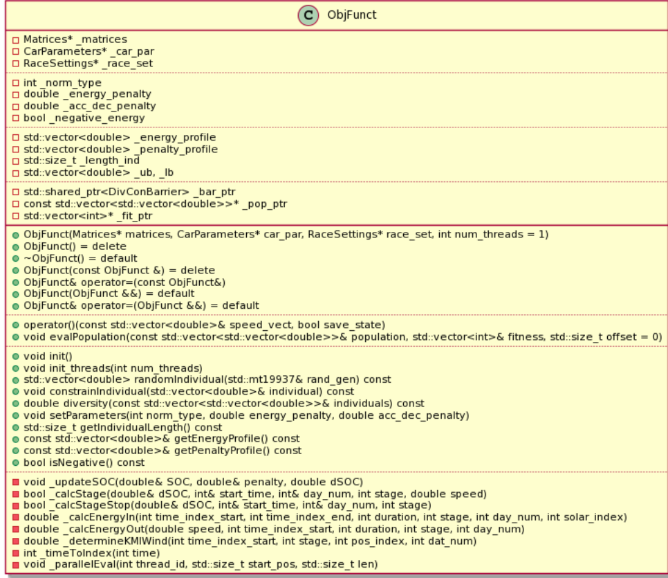
Figure 6.4: ObjFunc class diagram
