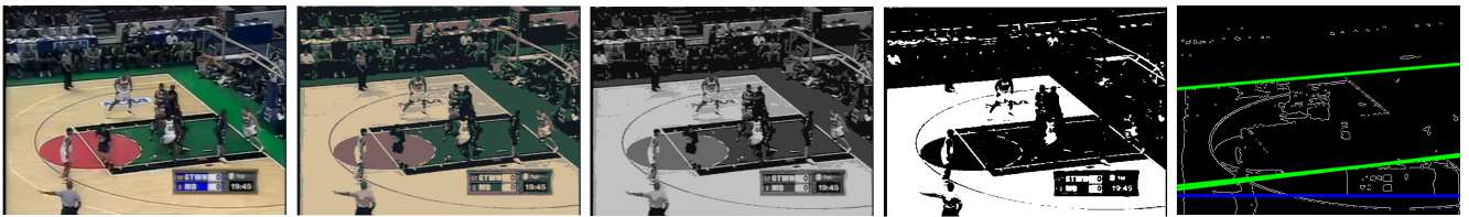
(b) Image is kept in RGB, k-means clustering is performed, all pixels colors are flattened to their cluster center, clustered image is turned to gray and thresholded.
