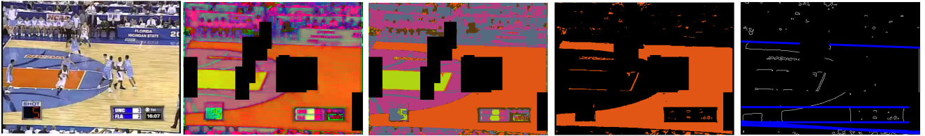
(a) Image is converted to HSV, k-means clustering is performed, non-dominant colors are blackened, pixels of dominant cluster are flattened to cluster center, bounding boxes are obscured.
