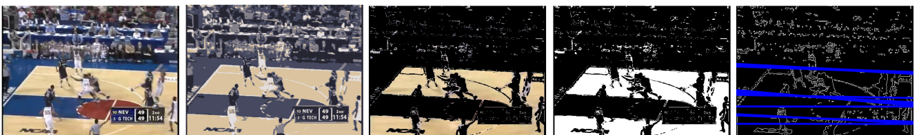
(c) Image is kept in RGB, k-means clustering is performed, non-dominant colors are blackened, pixels of dominant cluster keep their color, image is thresholded.
