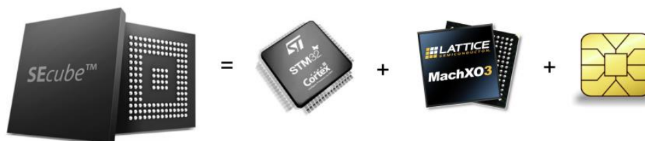
Figure 3.1.1. The components of the SEcube™ [9, p. 9].
