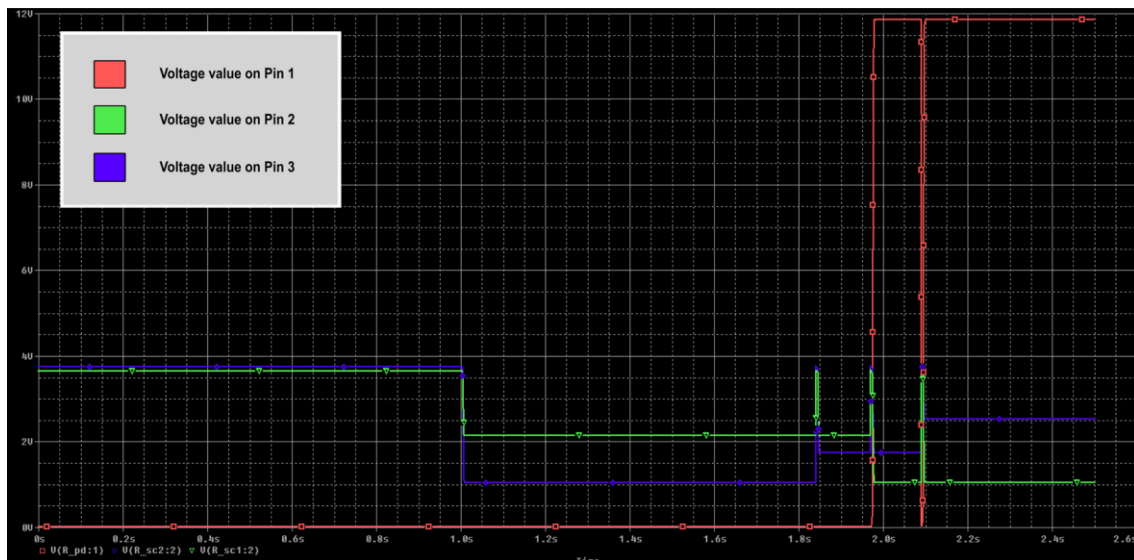
Figure 62: Simulated signals on pin 1 (red), pin 2 (green) and pin 3 (blue) in the configuration with Accessory
