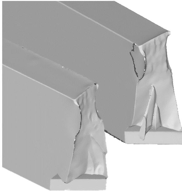
*Figure 5.4: Experimental crack surfaces of specimen 13467 with a strong factory roof effect*
