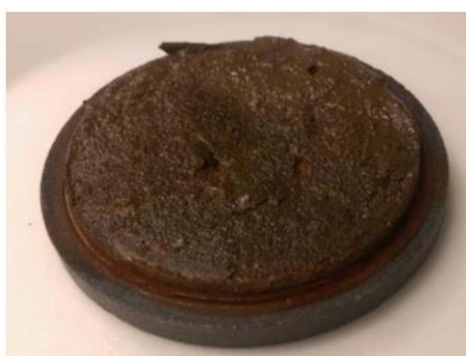
Figure 18 - Filter-cake of 120pcf fluid after treatment with 4%w/w HCl (Wagle, V. et al 2017a)
