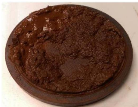
Figure 21 - Filter-cake of 120pcf fluid after treatment with a combination of 15%w/w formic acid precursor and 1% w/w HCl (Wagle, V. et al 2017a)
