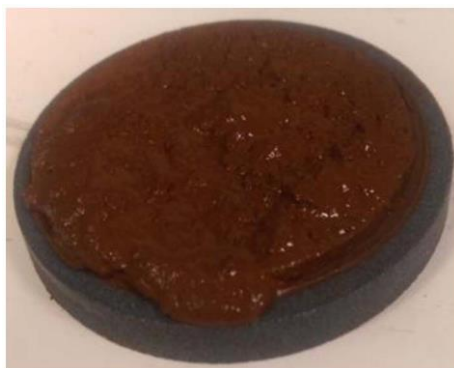
Figure 9 - Filter-cake of 100 pcf fluid after treatment with a combination of 15% w/w citric acid (Wagle, V. et al 2017b)
