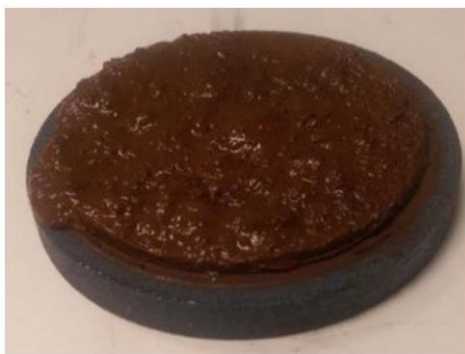
Figure 19 - Filter-cake of 120pcf fluid after treatment with 10%w/w glycolic acid (Wagle, V. et al 2017a)
