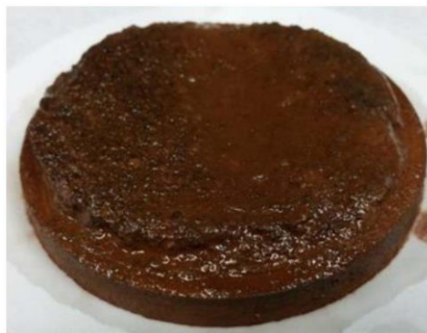
Figure 11 - Filter-cake of 100 pcf fluid after treatment with a combination of 15% w/w acetic acid (Wagle, V. et al 2017b)
