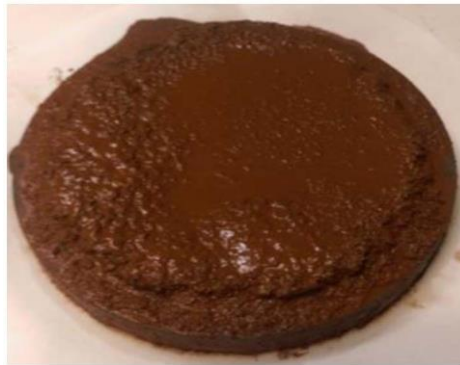
Figure 10 - Filter-cake of 100 pcf WBM after treatment with a combination of 15% w/w formic acid (Wagle, V. et al 2017b)
