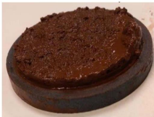
Figure 20 - Filter-cake of 120pcf fluid after treatment with 15%w/w formic acid precursor (Wagle, V. et al 2017a)
