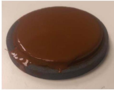
Figure 16 - Filter-cake of 120pcf fluid before any acid/acid precursor treatment (Wagle, V. et al 2017a)
