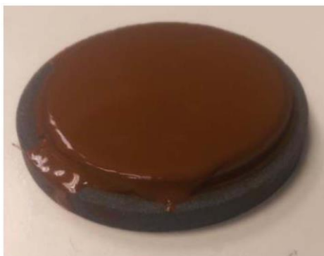
Figure 7 - Filter-cake of 100 pcf WBM before any treatment with aqueous organic acid (Wagle, V. et al 2017b)
