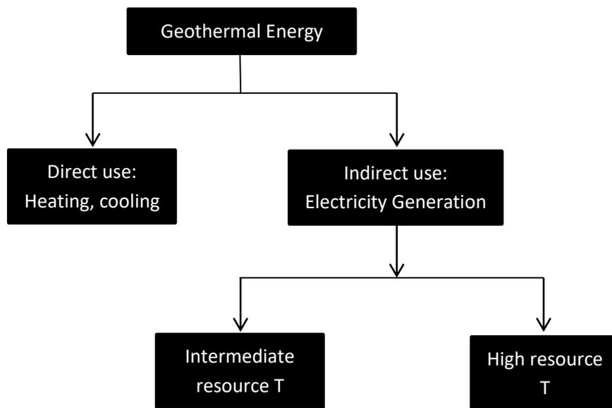
**Figure 2-General overview of geothermal energy resource**
