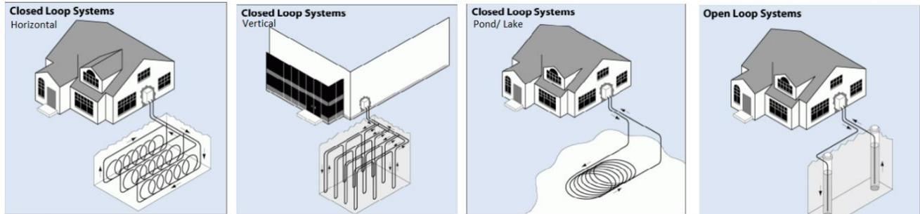
**Figure 4-Different configurations of GHPs**
