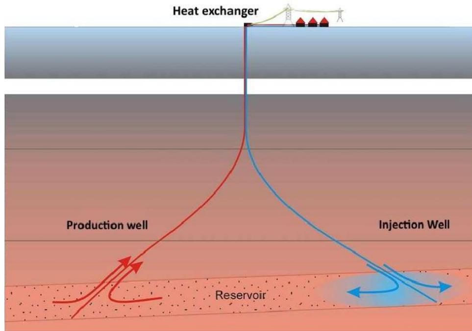
**Figure 3-General Layout of a geothermal doublet (T&A Energy, 2010)**
