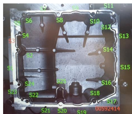
Figure 33. 2-Cylinders Gasoline engine's bead profile inspection results on the operator's monitor (oil sump processing workstation)
