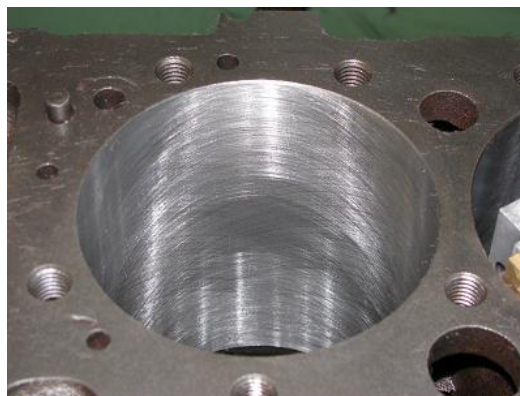
Figure 43. Crosshatch of a cylinder liner
