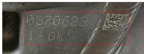
Figure 17. The diesel engine body's Data Matrix Code
