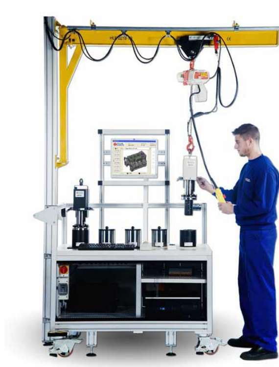
Figure 45. Gauging station for the cylinder liners' crosshatch: TAYLOR HOBSON Talys series
