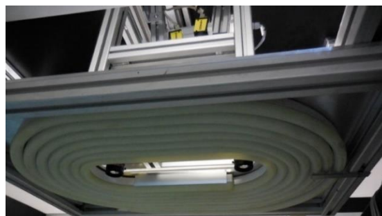
Figure 29. The cameras-lighting system in the silicone profile inspection stations on the Diesel engine's line
