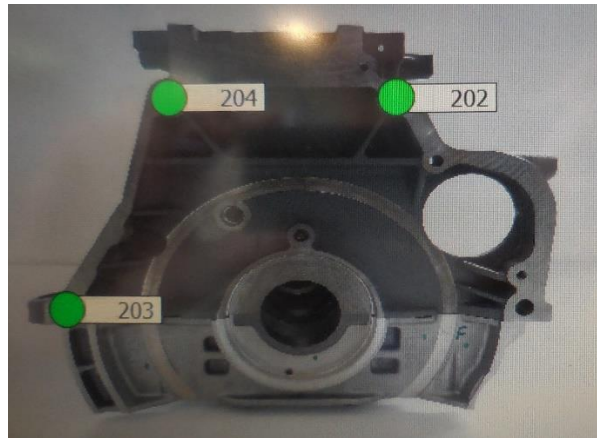
Figure 57. Final control on the machining line for the Diesel engine's body: Example of one of the four result windows shown on the operator's panel
