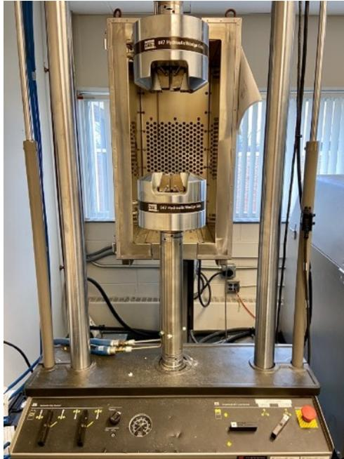
Figure 2.12 MTS 810 Material test system
