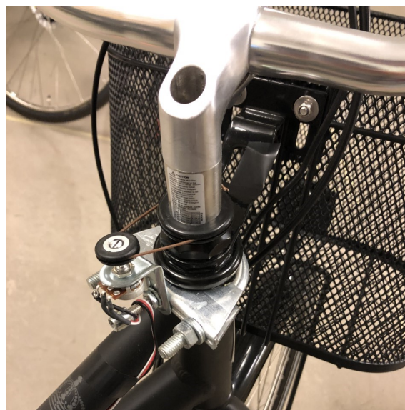
Figure 2.13: Steering angle sensor made with a potentiometer and a belt system
